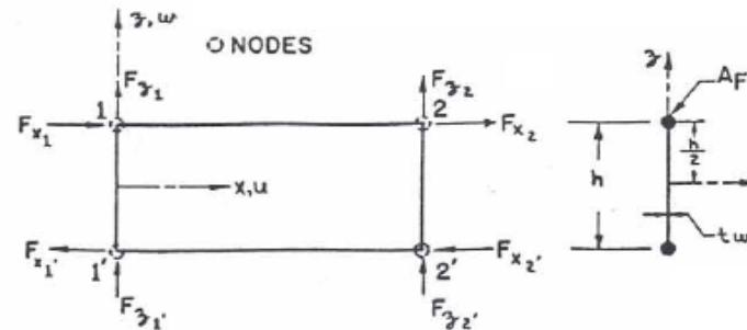
$$[K] = \frac{6EI}{Lh^2(1+4n)} \begin{bmatrix} u_1 & v_1 & w_1 & u_2 & v_2 & w_2 \\ (4/3)(1+n) & 0 & 0 & (4/3)(1+n) & 0 & 0 \\ 0 & -h/L & 0 & 0 & h^2/L^2 & 0 \\ -(h/L) & 0 & h^2/L^2 & 0 & 0 & h^2/L^2 \\ (2/3)(1-2n) & 0 & -h/L & 0 & 0 & 0 \\ 0 & 0 & 0 & 0 & 0 & 0 \\ h/L & 0 & -h^2/L^2 & h/L & 0 & h^2/L^2 \end{bmatrix}$$
