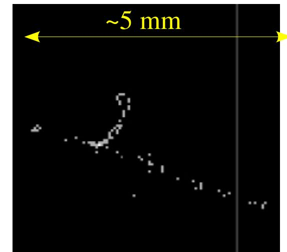
δ-electrons made visible in He/iC<sub>4</sub>H<sub>10</sub>,
