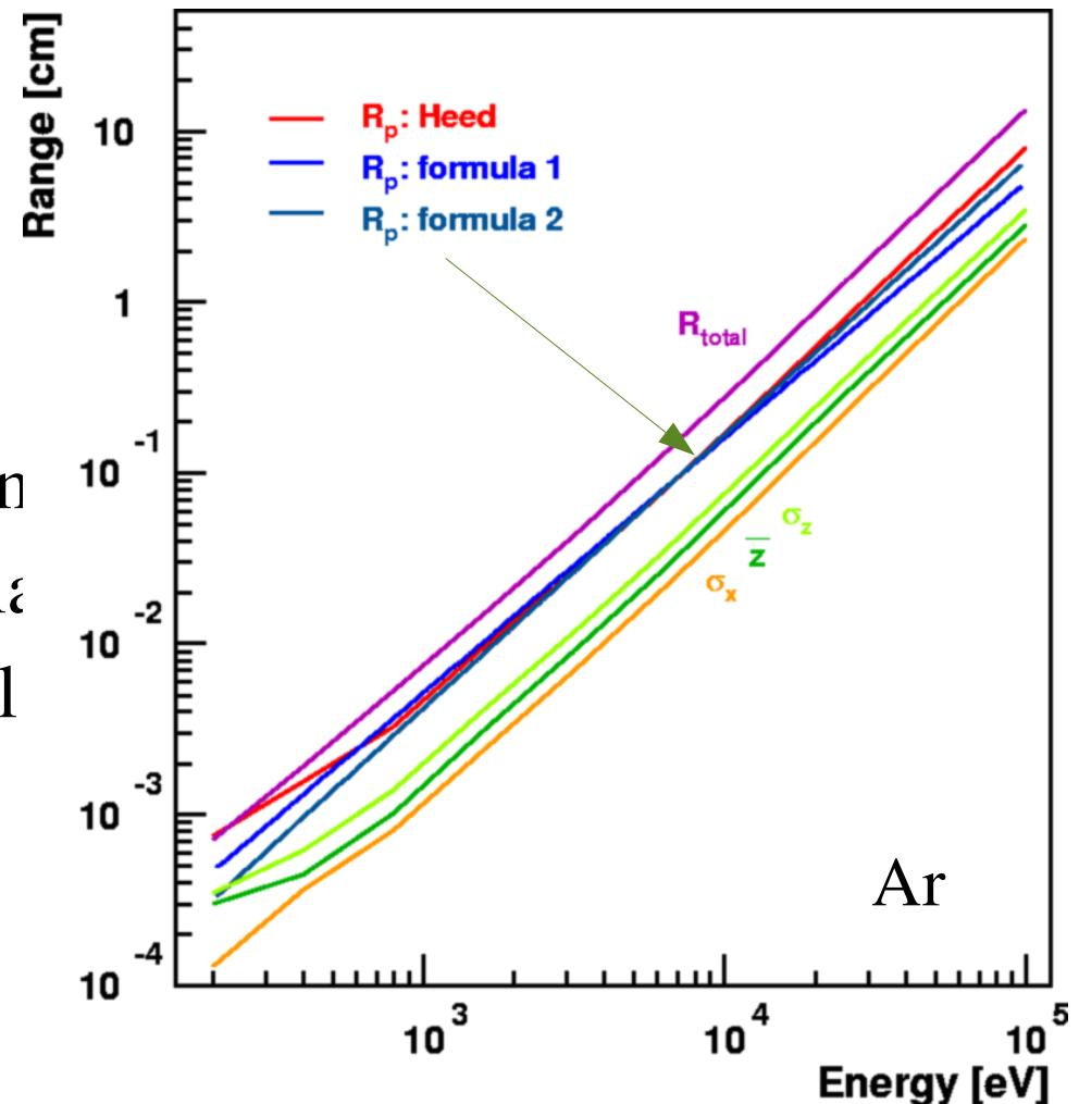
Practical range: distance at which the tangent through the inflection point of the descending portion of the depth-absorbed dose curve meets the extrapolation of the Bremsstrahlung background (ICRU report 35, 1984)
