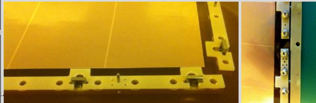
Easy to re-open detector for repair
