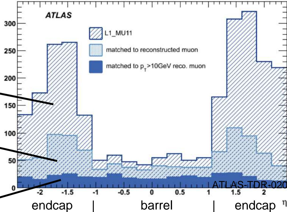
L1\_MU20 @  $3 \times 10^{34} / \text{cm}^2 \text{s} = 60$  kHz **Close to max. available 100 kHz** 5
