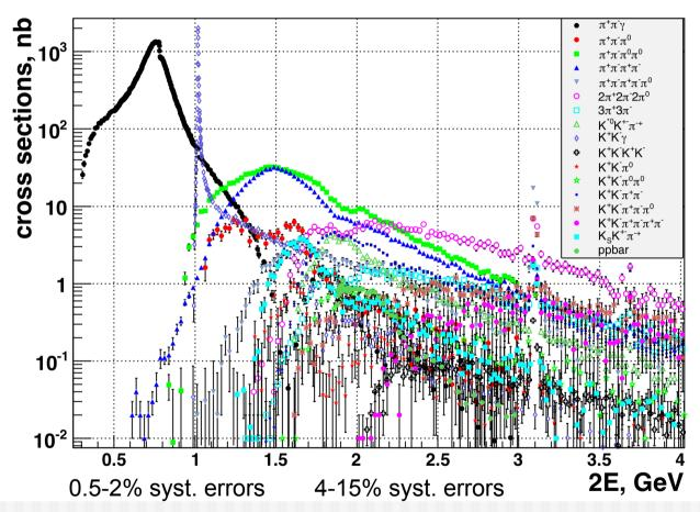
To calculate R in the energy range 1-2 GeV the processes  $\pi^+\pi^-3\pi^0,\,\pi^+\pi^-4\pi^0,\,K_SK_L,\,K_SK_L\pi^+\pi^-,\,K_SK^+\,\pi^-\pi^0$  are under study:  $\pi^+\pi^-2\pi^0$  will come soon. Work is in progress for  $K_SK_L\pi^0\pi^0,\,K_SK_L\pi^0$
