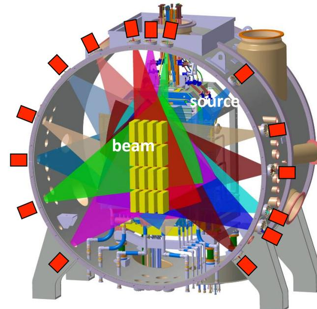
view of SPIDER vessel with 15 linear cameras of the tomographic diagnostic with corresponding lines of sight
