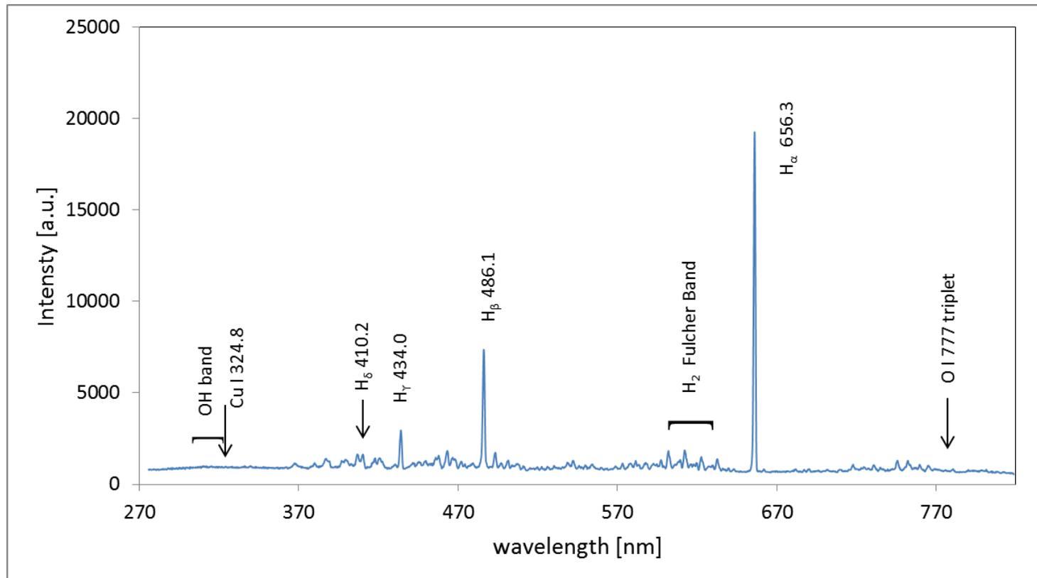
typical spectrum of the plasma light from the SPIDER Source, after several weeks of operation (pulse #5210). No visible traces of OH, Cu or O emission.
