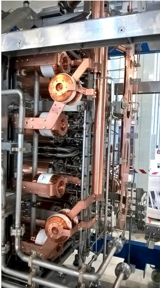
electrical connections and RF capacitors, gas injection and other auxiliaries on the upstream side of the source
