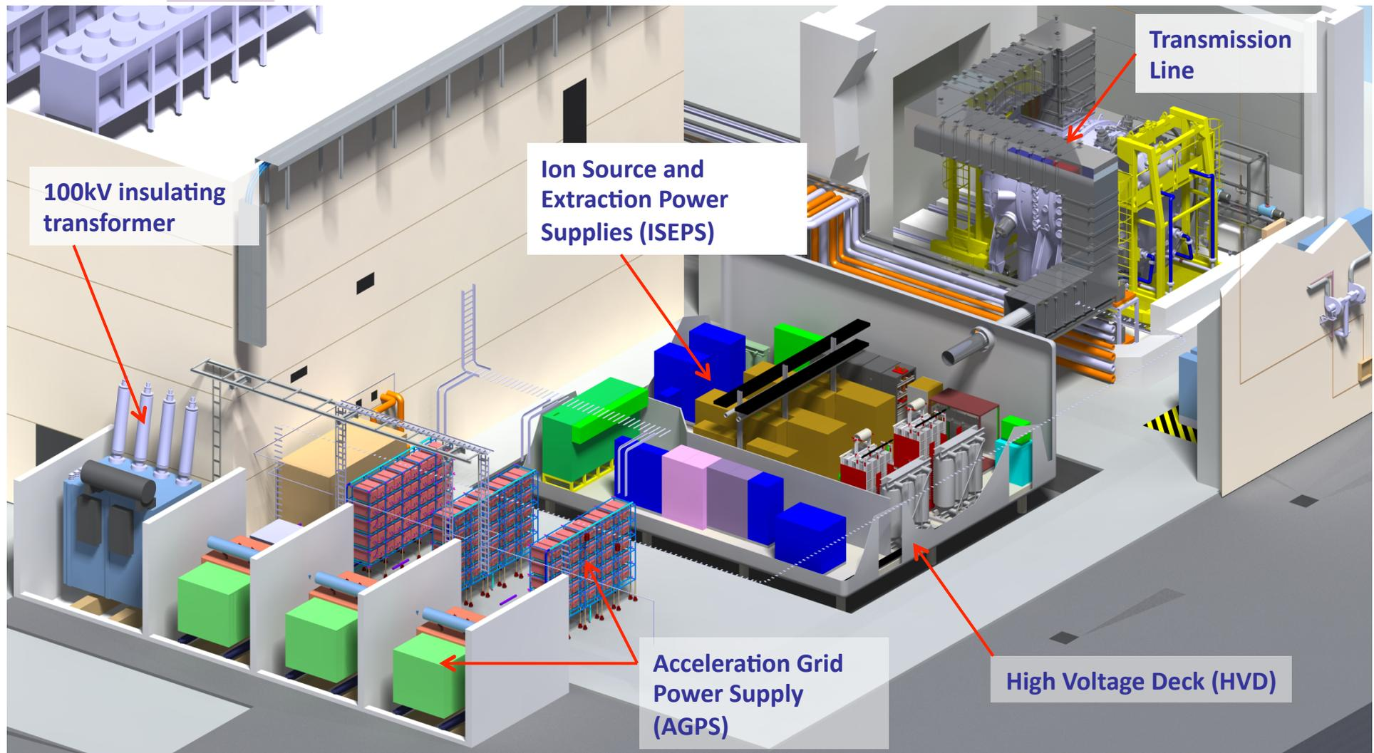
3D CAD view of SPIDER Power Supply, TL and Vessel
