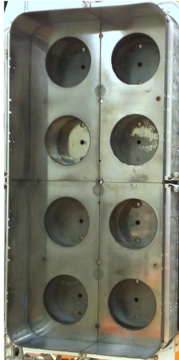
Plasma Source chamber with 8 RF drivers during assembly
