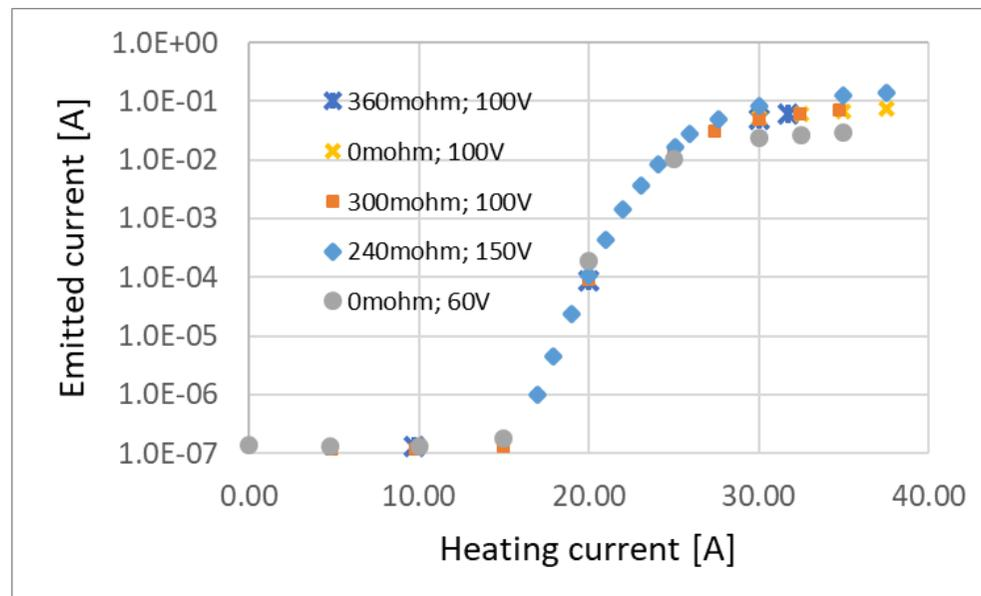
Current emitted by pre-ionisation filaments as a function of the heating current in different conditions
