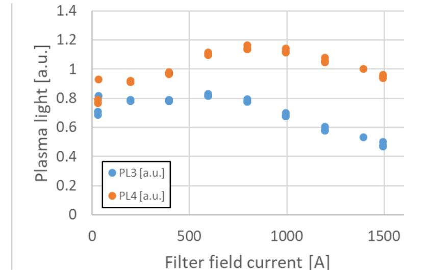
Plasma light from drivers #3 and #4 as a function of the filter field current.
