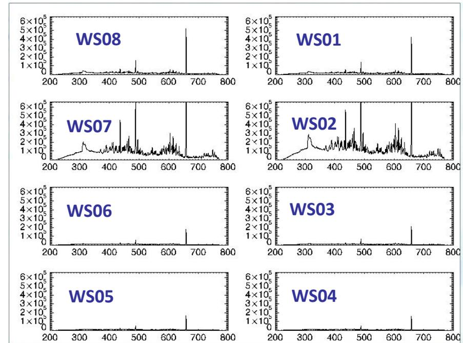
Plasma light spectra measured through the RF drivers, only drivers #3 and #4 are powered
