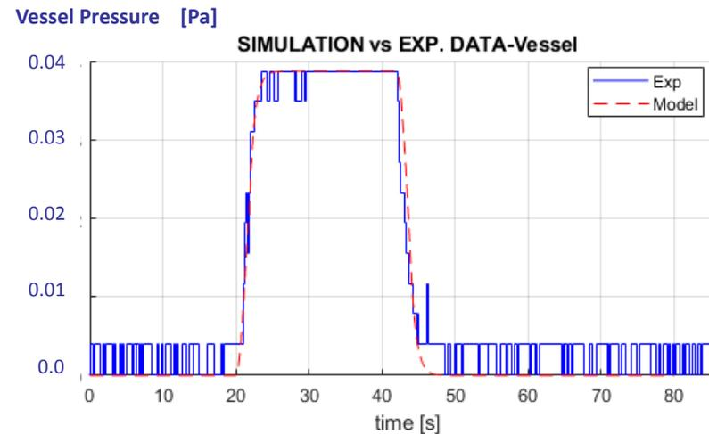
source and vessel pressures measured by capacitive sensors are in fairly good agreement with numerical dynamic models
