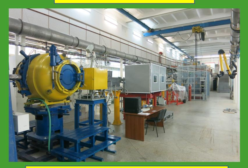
Source - wiggler, B = 1.2 T (7-pole),  $E_{el} = 4 GeV$ ,  $I_{el} = 10 mA$
