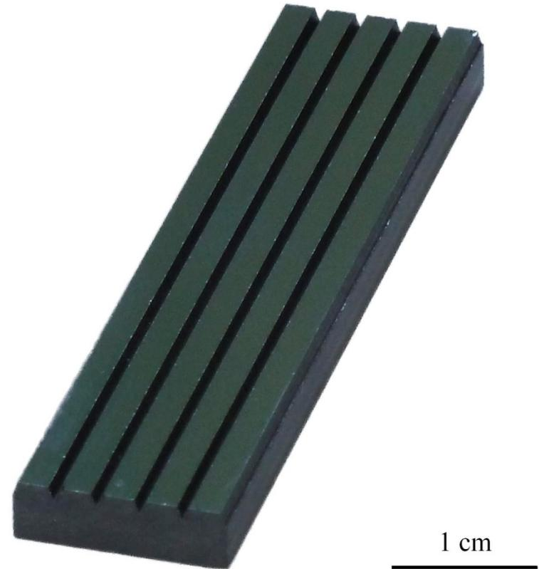
Photo of a silicon wafer with grooves.
