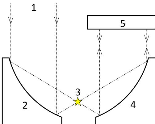
**Quasi-continuous terahertz laser discharge and optical scheme of negative optical feedback for its stabilization:**
