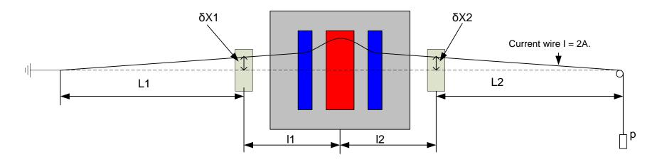
$$I_{first} = I_1 \left(\frac{L}{2}\right) = \delta \alpha * \frac{T}{I} = \frac{T}{I} \left(\frac{\delta x 1}{L1} + \frac{\delta x 2}{L2}\right) \text{-first field integral}$$
