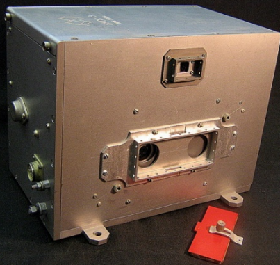
Solar UV radiation sensor VUSS-E Fedorov IAG, Moscow
