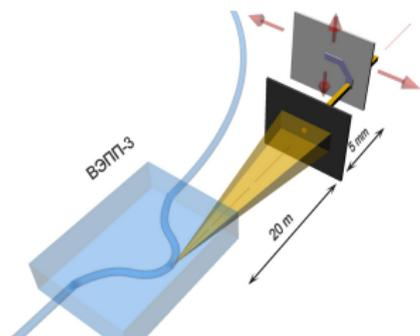
Preliminary opening, which limits the irradiation field, and an X-ray mask with a microopening of 15 to 60 microns in size are installed in the SR beam. The shape of microopenings on the mask is variable. Combining a microopening with a pre-opening yields a pencil beam of required size. Using such a pencil beam and moving the  $XY\Phi$  stage, one can draw directly on a thick layer of high-sensitivity resist.
