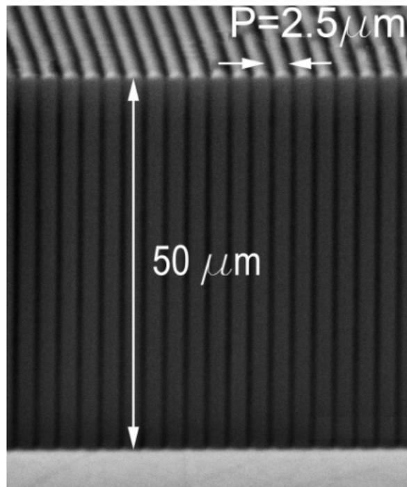
Fragment of grating of SU-8 resist. Exposure was at "LIGA" station with beamstop.
