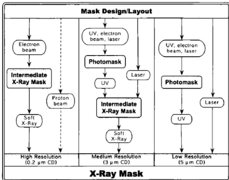
Figure: Overview of X-ray mask fabrication methods. Y. Desta and J. Goettert. X-ray Masks for LIGA Microfabrication. In *Advanced Micro & Nanosystems Vol. 7. LIGA and Its Applications*, page 28, 2009
