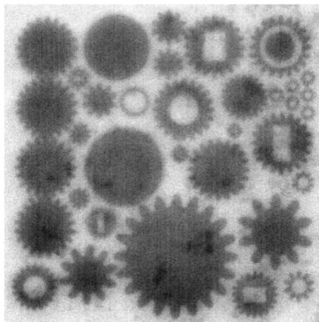
Images of X-ray mask patterns recovered at the X-ray microscopy station. Photon energy 6 keV. At figure a) outer ring have linewidth  $20 \mu\text{m}$
