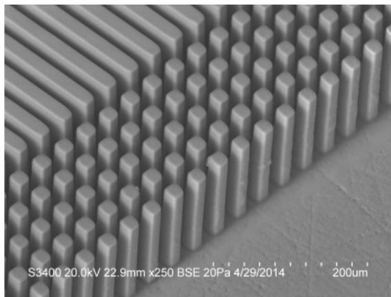
SU-8 microstructures, thickness is about  $100 \mu\text{m}$ . Width of pinches is  $20 \mu\text{m}$ , period is  $40 \mu\text{m}$
