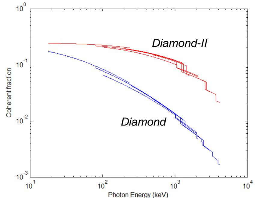
The improvement in brightness/coherence is approximately a factor of x3 at 100 eV x10 at 1 keV, x12 at 10 keV, the main benefit coming from the reduction in horizontal source size
