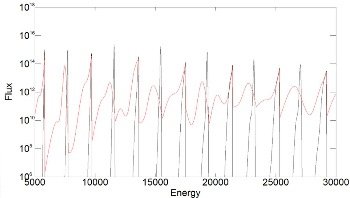
*Flux through a  $40 \mu\text{rad} * 40 \mu\text{rad}$  aperture for the CPMU in the existing ring (red) and in Diamond-II (black).*
