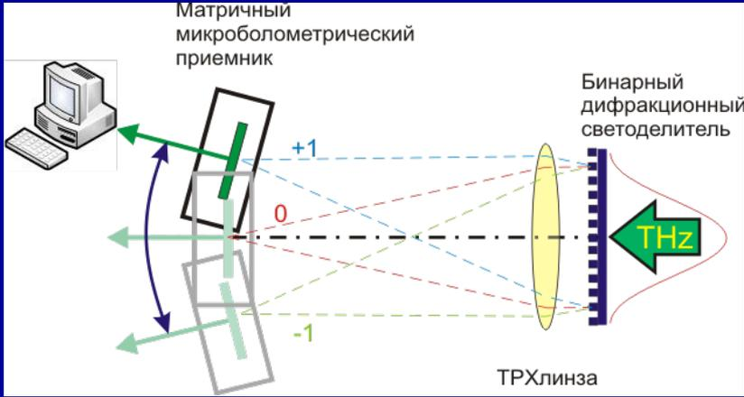
Experimental investigation of DOEs at free electron laser - NovoFEL.
