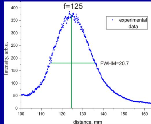
Measured intensity distribution along optical axis
