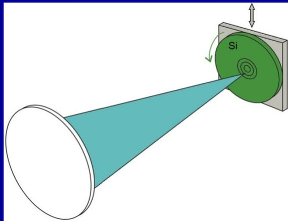
Scheme of laser ablation ( $\lambda = 1030$  nm,  $\tau = 400$  fs,  $f = 200$  kHz, Yb:YAG laser) of silicon plate
