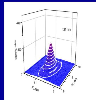
3D intensity distribution at different distances from fabricated lens (focal distance is 125 mm)
