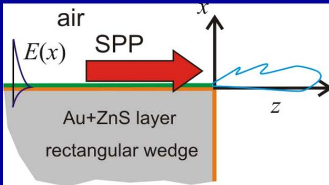
Registration of plasmon-polariton by use of diffraction at the waveguide wedge
