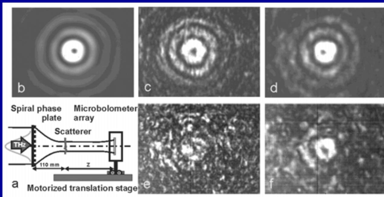
Selfreconstruction of Bessel beams. (a) Scheme of experiment. (b) Beam cross-section  $z=110$  mm. Beam after scatterer (thin film): (c)  $Z = 60$  mm, (d)  $Z = 115$  mm. Beam after scatterer (thick film) : (e)  $Z = 60$  mm, (f)  $Z = 115$  mm.
