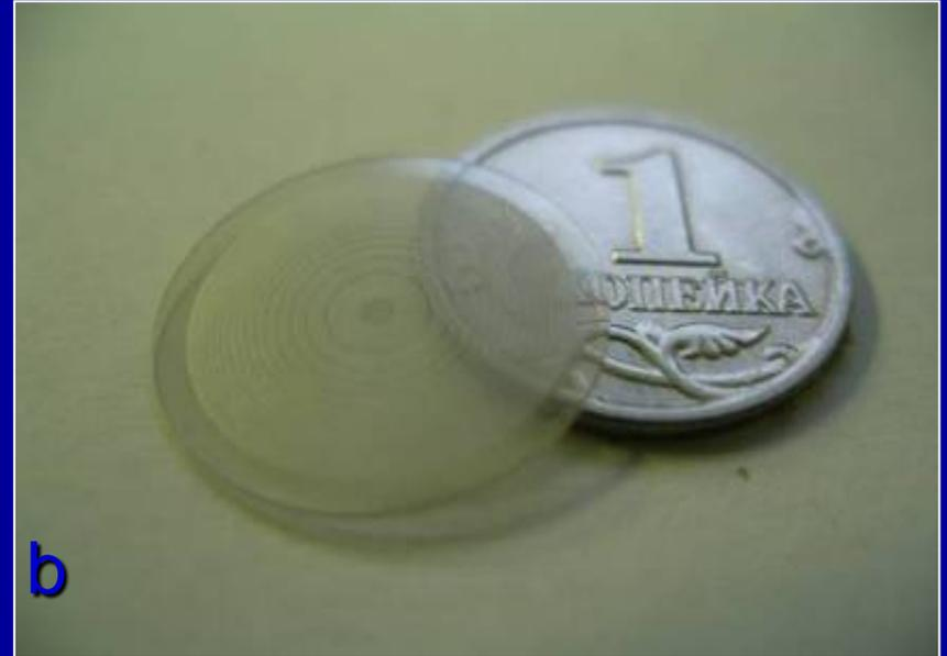
Diamond diffractive lens before (a) and after (b) removing of graphite
