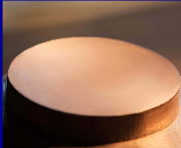
3-D printing + vacuum deposition of copper layer
