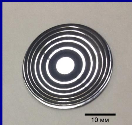
Fabricated 4-level diffractive lens
