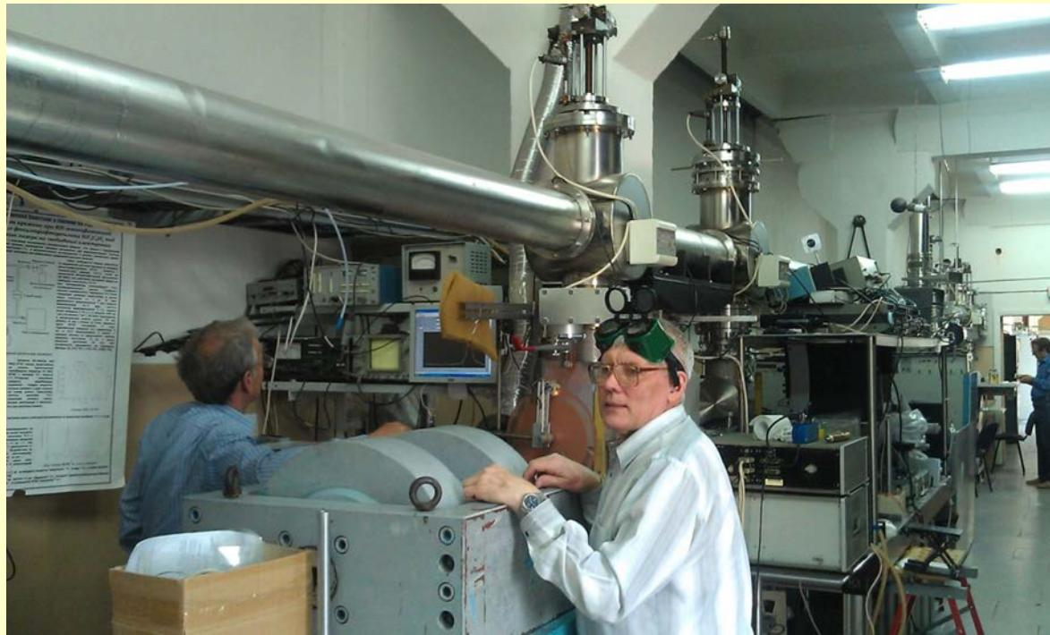
The station is equipped with grating monochromator, various optical gas cells and optical elements, electromagnet and solenoids for Zeeman and Faraday experiments. There are also pulsed CO<sub>2</sub> and N<sub>2</sub> – lasers, synchronized with FEL.
