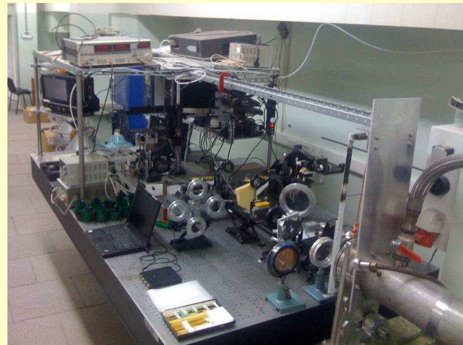
**Multifunctional station equipped with an optical table (3x1.5 m), large variety of optical elements, one-channel and imaging sensors, helium cryostat, high-speed oscilloscopes, lock-in amplifiers, home-made THz ellipsometer, THz interferometers, etc.**
