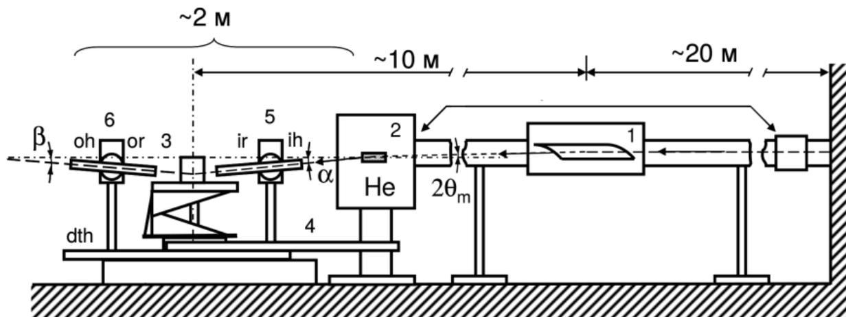
1 – thoroidal X-ray mirror; 2 – single-crystal monochromator; 3 – vibro-damping platform and sample chamber; 4 –  $2\theta$ -rotation platform; 5 – two-slit collimator; 6 –  $\beta$ -rotation platform with detector slit.
