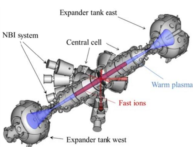
**FIGURE 1.** The layout of GDT experiment.
