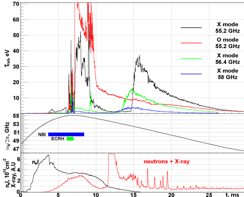
FIGURE 4. ECE radiation temperature, magnetic field at the GDT axis, X-ray signal and linear plasma density in the discharge with combined NBI and ECRH plasma heating.
