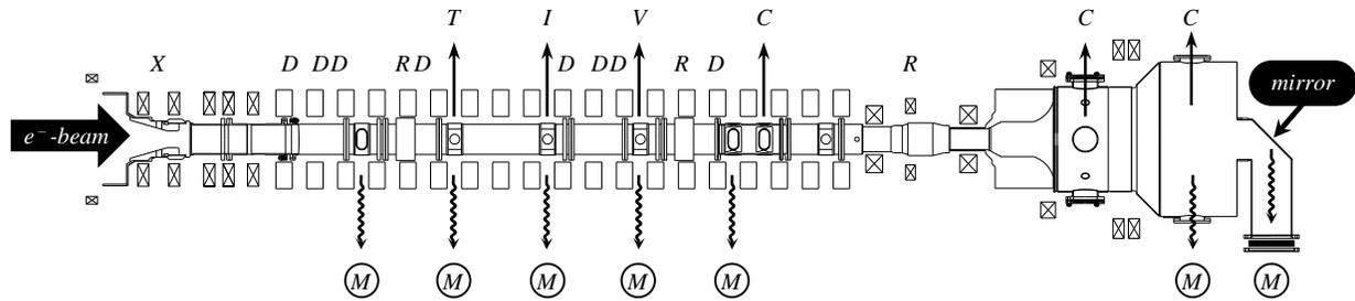
**FIGURE 1.** Scheme of the location of different diagnostics at GOL-3T facility. *X* – detectors of hard X-ray; *D* – diamagnetic loops; *R* – Rogowski coils; *C* – CCD-cameras; *V* – vacuum ultraviolet detector; *T* – Thomson scattering; *I* – Michelson interferometer; *M* – detectors of subterahertz radiation. Radiation propagating along the axis is measured via rotary metal mirror.
