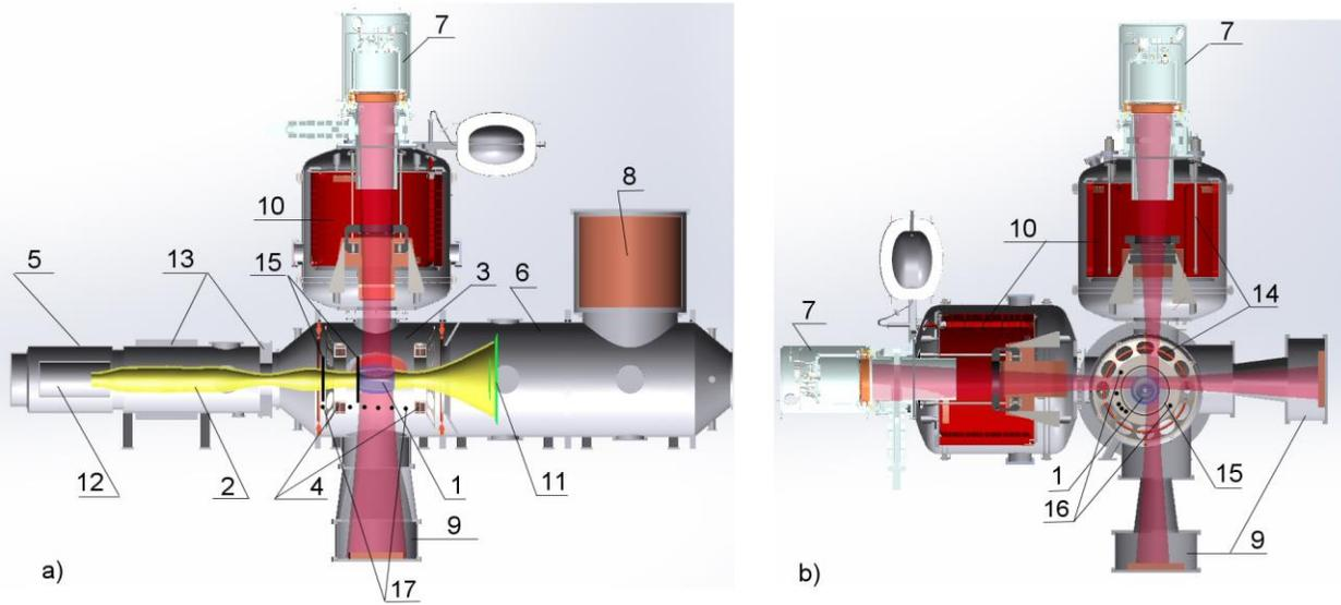
**FIGURE 1.** The CAT layout: a) Longitudinal section of the experimental setup, b) the cross-section in the middle plane.
