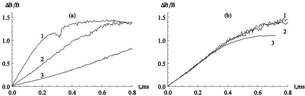
**FIGURE 2.** Time dependence of ratio between diamagnetic field perturbation and vacuum magnetic field at different target plasma densities (a) and electron temperatures (b) determined from PiC simulations [3]. Injection energy 15 keV, neutral beam current 240 A. Target plasma density: 1 –  $n_e=10^{14}\text{cm}^{-3}$ , 2 –  $n_e=3\cdot 10^{13}\text{cm}^{-3}$ , 3 –  $n_e=10^{13}\text{cm}^{-3}$ . Electron temperature: 1 –  $T_e=100\text{eV}$ , 2 –  $T_e=50\text{eV}$ , 3 –  $T_e=30\text{eV}$ .
