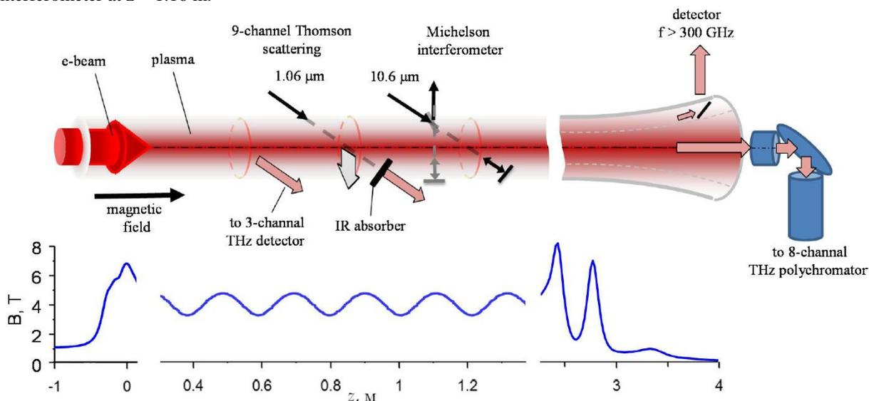
**FIGURE 1.** Layout of the GOL-PET device with the diagnostics (top). The longitudinal confining magnetic field distribution is presented on the bottom of figure. Here the multiple-mirror configuration is shown. In the uniform configuration the central part of the diagram one need to replace to flat curve.
