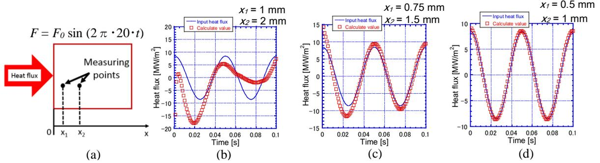
**FIGURE 5.** (a) The schematic view of calorimeter model. (b) Calculation result in the case with  $x_1 = 1$  mm,  $x_2 = 2$  mm. (c) Calculation result in the case with  $x_1 = 0.75$  mm,  $x_2 = 1.5$  mm. (d) Calculation result in the case with  $x_1 = 0.5$  mm,  $x_2 = 1$  mm.
