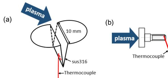
**FIGURE 2.** (a) The schematic of calorimeter in V-shaped target. (b) The schematic of calorimeter near the target.
