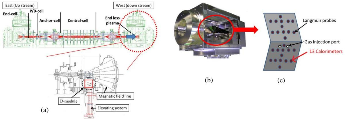
**FIGURE 1.** (a) GAMMA 10/PDX. (b) The picture of D-module. (c) Target plate.
