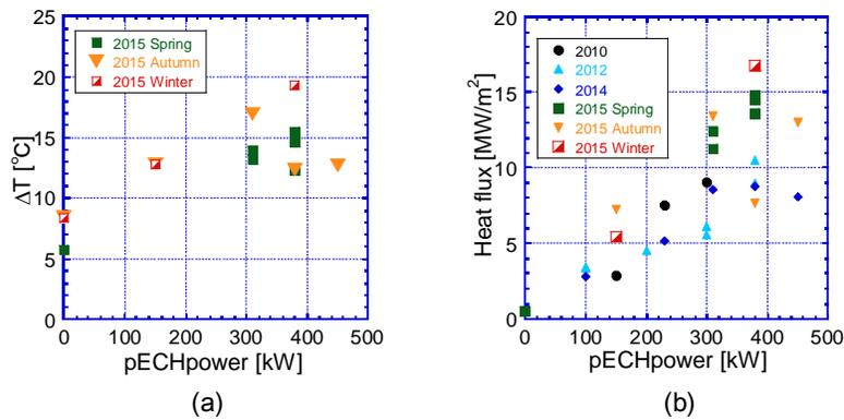
FIGURE 4. (a) Heating power dependence of temperature differences. (b) Heating power dependence of heat flux.
