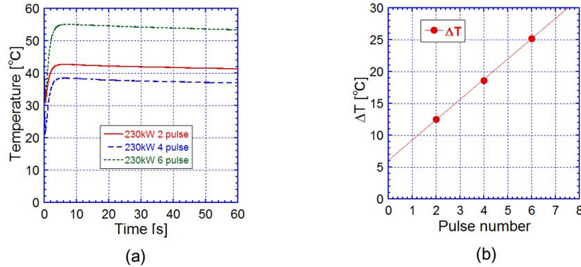
FIGURE 3. (a) Time dependence of substrate temperature. (b) Heating time length dependence of temperature increment.
