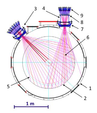
FIGURE 1. Layout of the optical 2D tomographic diagnostic: 1 – cross section of the vacuum vessel of the plasma installation, 2 – plasma boundary, 3 – "WIDA-diameter" bundle, 4 – "WIDA-radius" bundle, 5 – line of sight, 6 – area of best accuracy of tomographic reconstruction, 7 – two-axis angular aligning unit, 8 – measurement module holder with temperature stabilization, 9 – three-channel standard measurement module.
