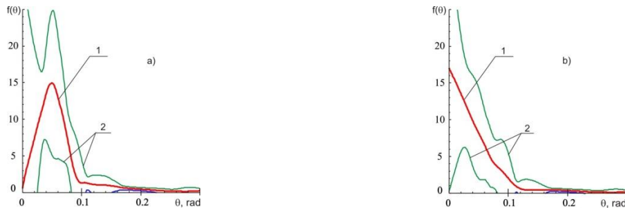
FIGURE 4. 1- angular distribution function, 2- strip of events for two cases: a) the detector axis is parallel to the magnetic field, b) it was inclined at the angle 2 mrad
