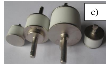
FIGURE 9. Thyatron drivers for TDI, TPI and TGI-switches
