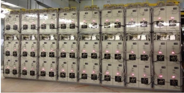
FIGURE 2. Pulse generators of linear accelerator LIU-2 is an assembly of 48 modulators with TPI2-10k/50 thyratrons
