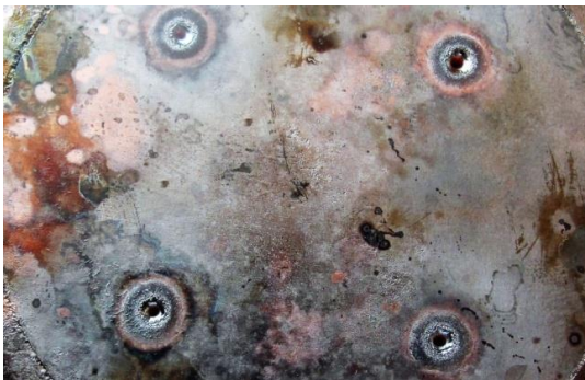
FIGURE 1. Arc drilling in anode of TDI1-50k/25 switch, operated in the following mode: U_a = 20 kV, frequency = 200Hz, peak current 7 kA, \tau = 1.5 \mu s, Q=10 mC per shot, leading edge 100 ns.
