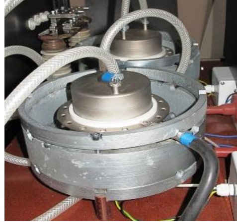
FIGURE 6. Assembly of two water-cooled thyratrons TDII-200k/25HW with hollow anodes, operating in parallel in high-power pulsed plasmatron pulser [5]. The thyratrons switch 1.2 mF (up to 20 kJ per shot) at average current 10 A. The switches are placed into steel tubes – shields with thickness of 10 mm, consisting of 3 parts.
