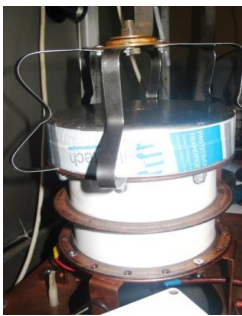
FIGURE 9. Thyatron TD11-150k/50H with a screen in the test facility (from the left). Screen photos (inside view).
