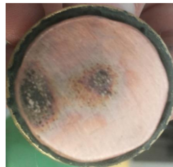
FIGURE 14. Arc traces without shield after multiple shots with current amplitude up to 5 kA.
