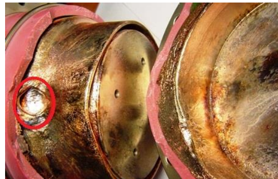
FIGURE 2. Image of electrodes in thyatron TDI1-150k/25 after arcing.
