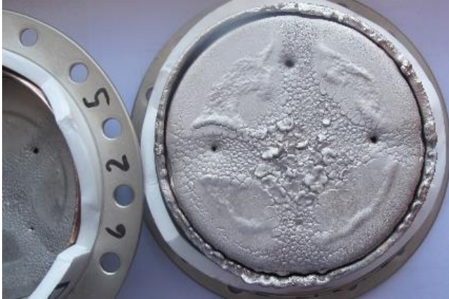
FIGURE 3. Traces of erosion of the cathode surface when of symmetrization current leads on the flange circumference
