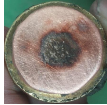
FIGURE 16. Arc traces with a ferromagnetic shield after multiple shots with current amplitude up to 5 kA.
