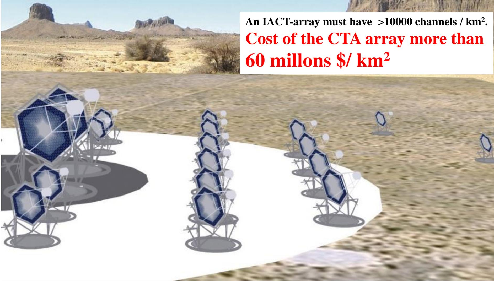
An IACT-array must have  $>10000$  channels / km<sup>2</sup>.
