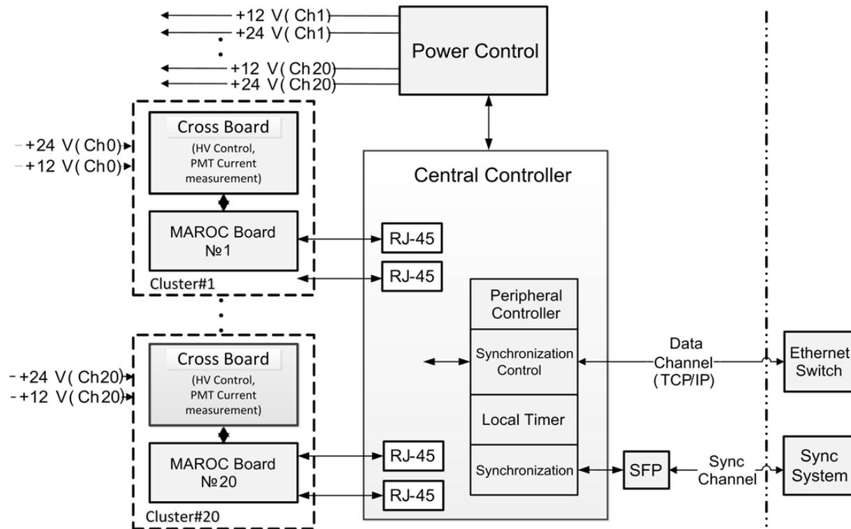
controls of the PMT board operation (setting the high voltage and monitoring the PMT current), the common trigger formation, the PMT cluster data collection, synchronization, storage of data in the intermediate buffer, and the traffic of data between data collection centers and the Controller via Ethernet.
