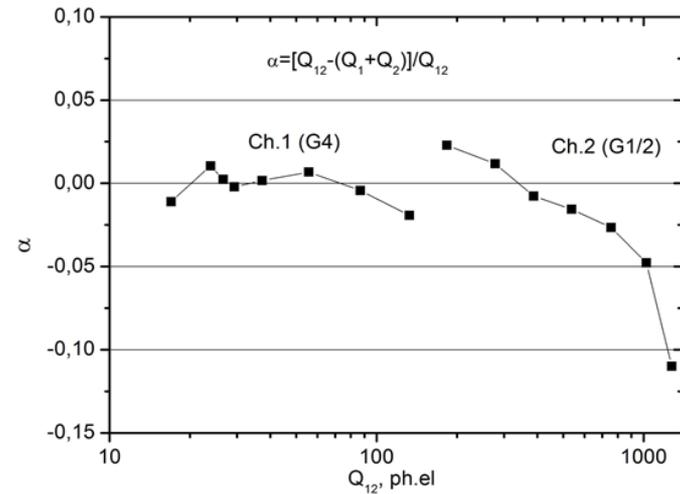
The linearity of the single spectrometric channel
