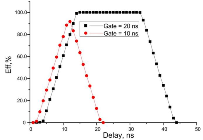
Dependence of the first level trigger formation efficiency on the delay.
