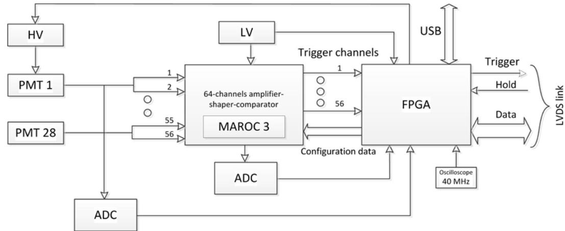
Two channels of MAROC3 process the signals from one PMT spited to provide the necessary dynamic range.
