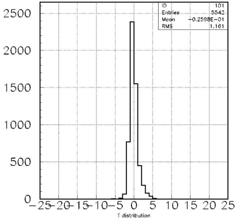
The **RMS=1.1 ns** for TAIGA-HiSCORE provides an accuracy of an  $\gamma$  and CR arrival direction about **0.1 degree**
