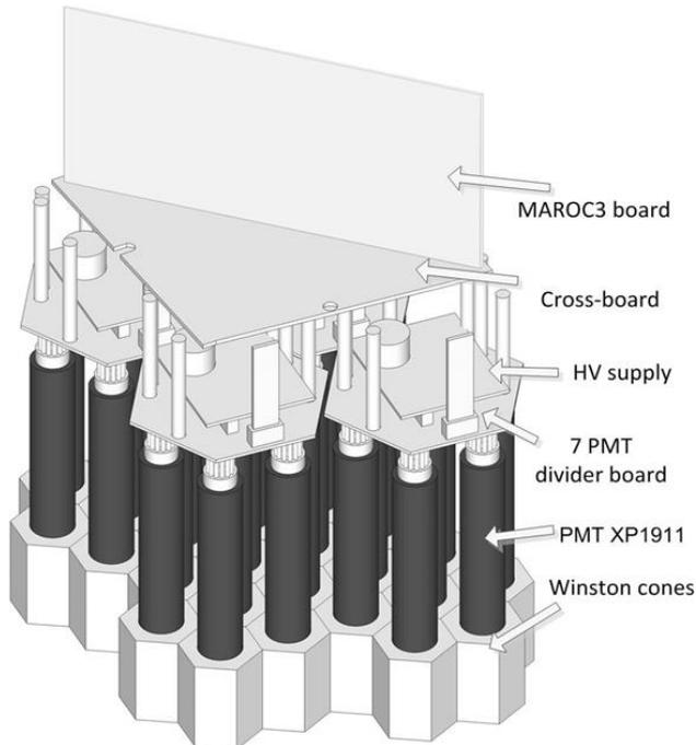
Basic cluster: 28 PMT-pixels arranged in four hexagonal cells 7HEX. The shaded area: the cross-board plate. Signal processing: PMT DAQ board based on the MAROC3 ASIC
