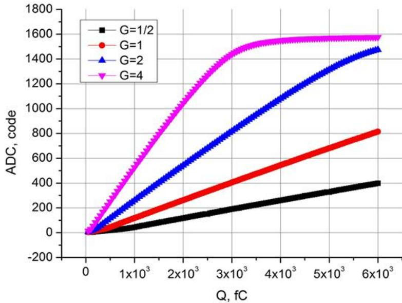
Calibration characteristics of a spectrometric channel of the ASIC MAROC3 for different preamplifier transmission coefficients.
