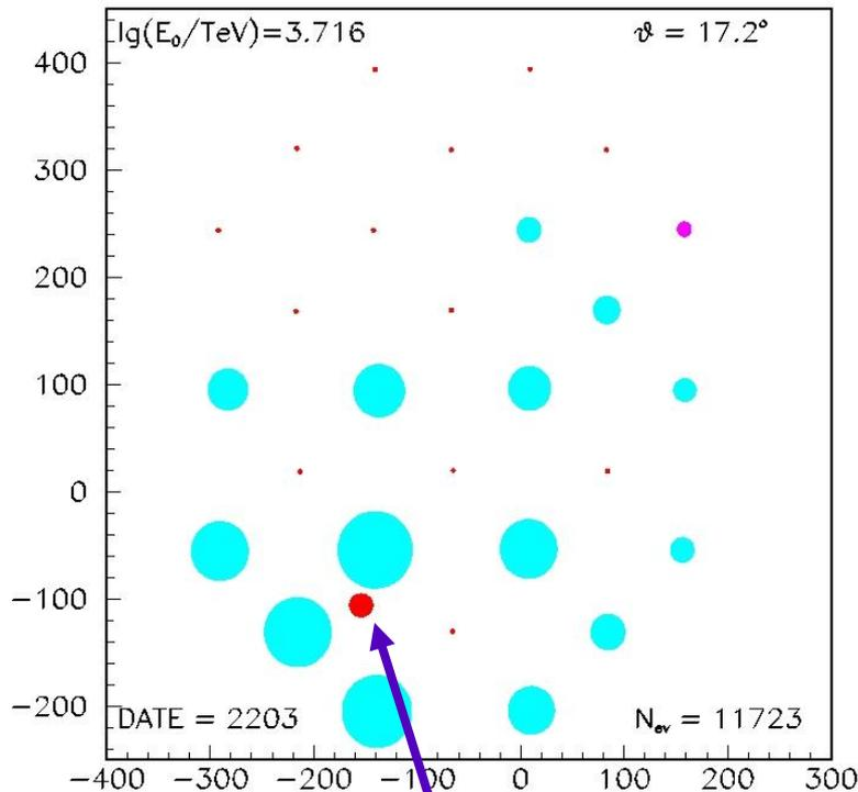
Reconstructed core position for an event, the area of the circles is proportional to  $\log A$ , with  $A$  the station signal amplitude
