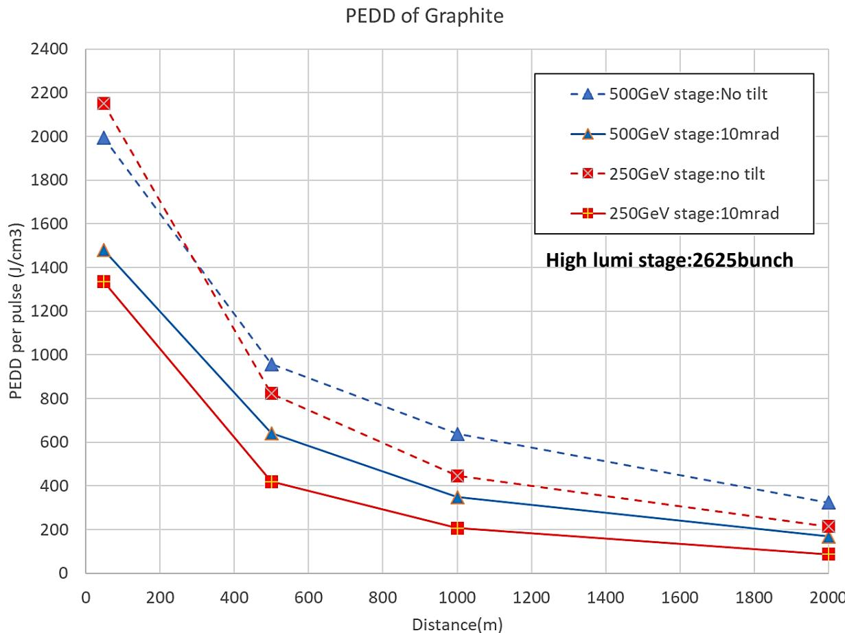
\* Distance : from Positron Target to Dump
