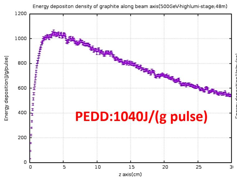
Energy depositon density of graphite at peak energy deposition density(500GeV-highlumi-stage;48m)
