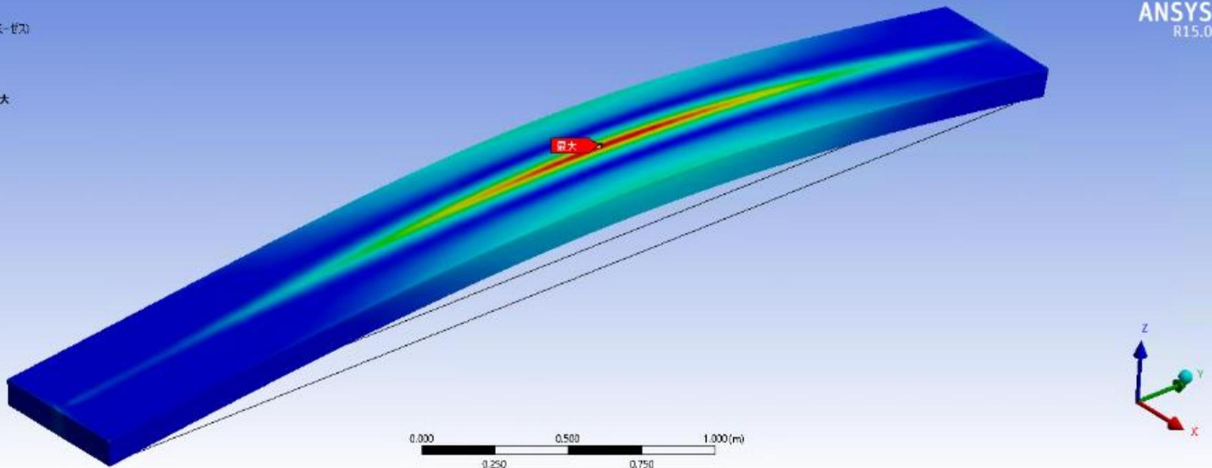
Max Von Mises stress of Copper-plate : **138MPa**
