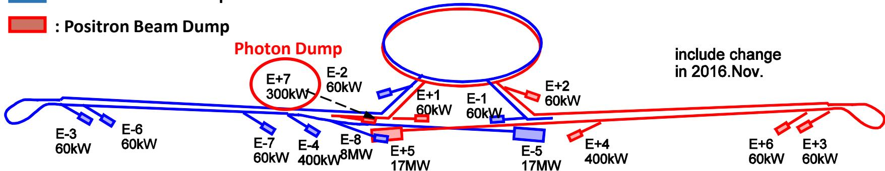
**Total 15 Beam dumps in ILC . Beam dumps are classified into 5 types.**
