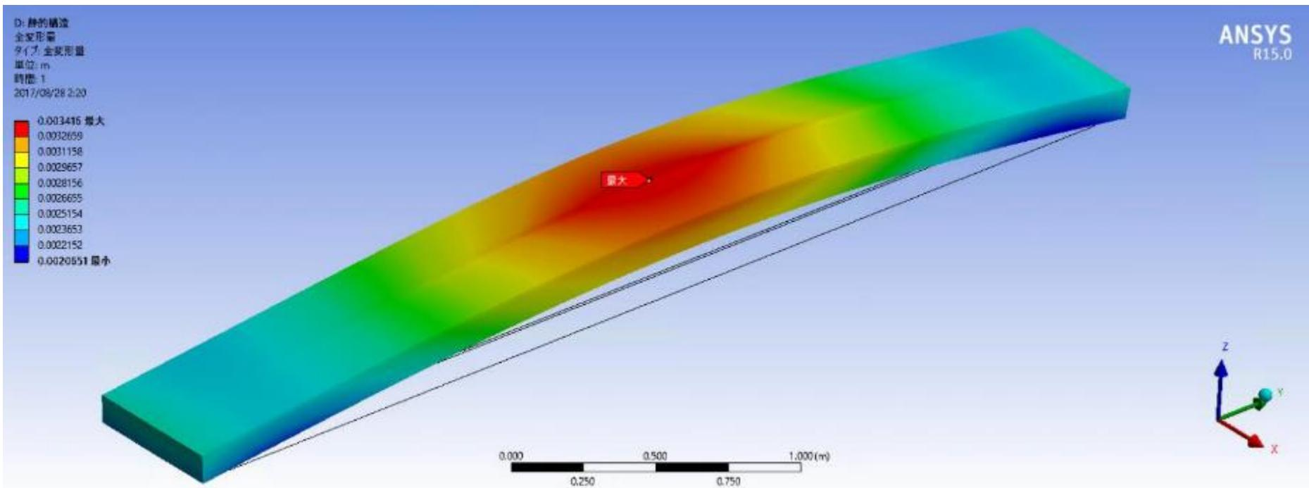
Main plate is expanded and main plate is arched **3.4mm** in the surface direction
