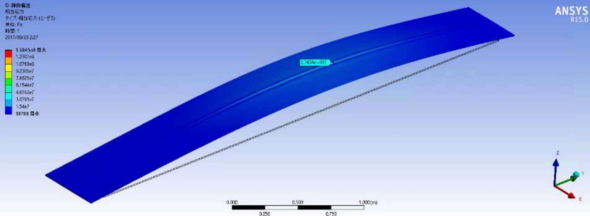
Max Von Mises stress of Graphite-plate : **27MPa**
