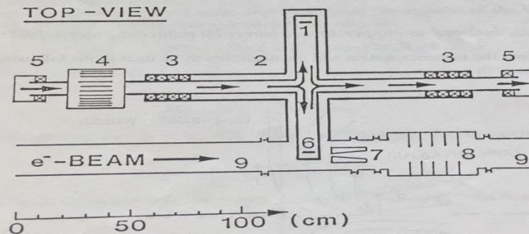
KEY: 1: Target Wheel. 2: Vacuum Tank. 3: Rotating Vacuum Feedthrough. 4: Motor.
