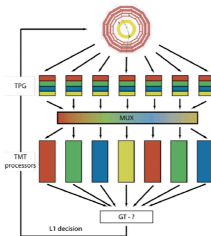
transition from parallel triggering systems to *time-multiplexed trigger*
