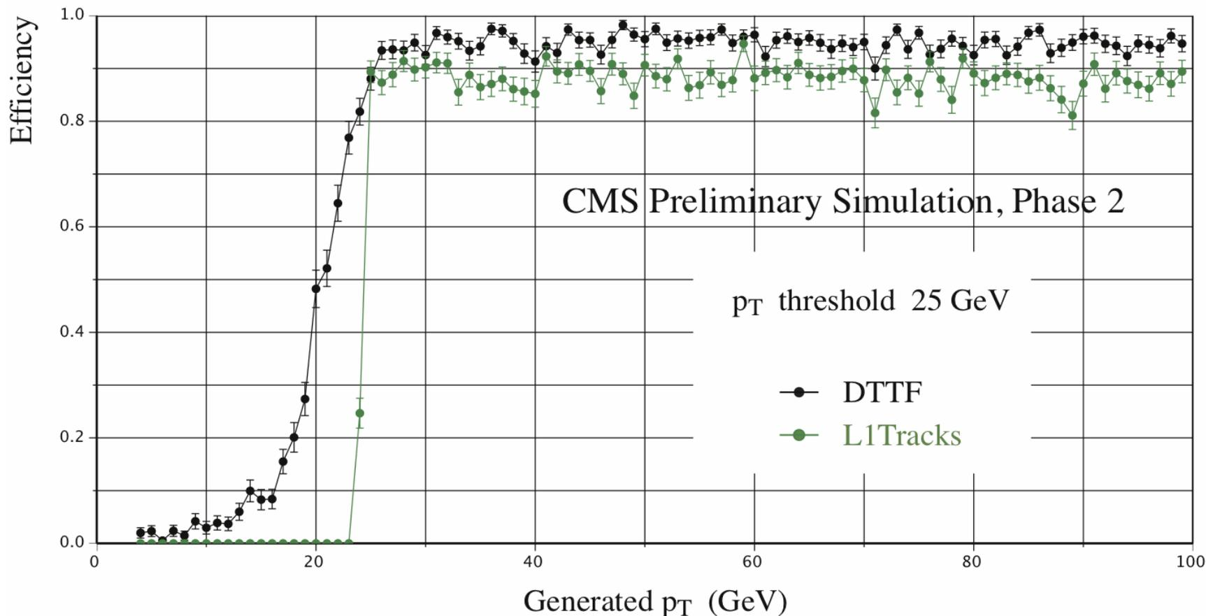
Much sharper turn-on curves w.r.t. DTTF, as expected from the much better  $P_T$  resolution. Hence the contribution from mis-measured low  $P_T$  muons (which makes most of the DTTF rate) is dramatically reduced.
