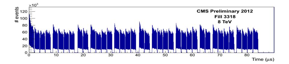
Bunch structure of one full orbit inside LHC, abort gap on the right
