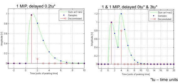
Identify pulse arrival time and peak height, distinguish signals close in time (overlapping) "deconvolution"
