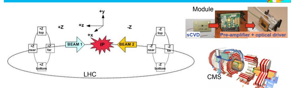
8 single-crystal CVD diamonds (5 \* 5 \* 0.5 mm<sup>3</sup>, Element 6) positioned around the beam-pipe, radial distance 4.5 cm, 1.8 m from interaction point
