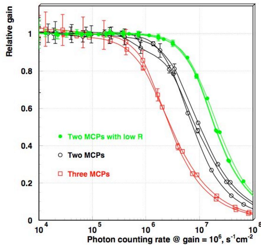
MCP with low resistivity can provide counting rate capability up to several MHz/cm<sup>2</sup>
