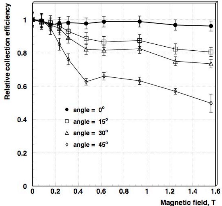
Collection efficiency does not change in axial magnetic field
