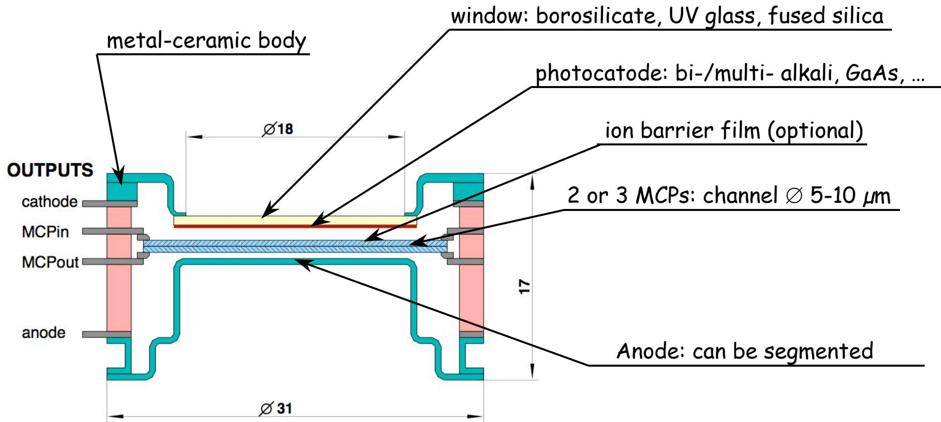
Transfer method: photocathode and MCPs are prepared separately and then assembled in ultra high vacuum.
