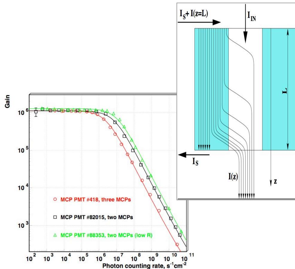
Gain decreases when output current becomes comparable with MCP strip current
