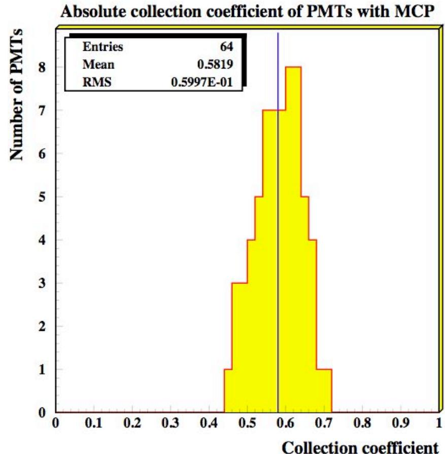
Photoelectron collection efficiency  $\approx 0.6$
