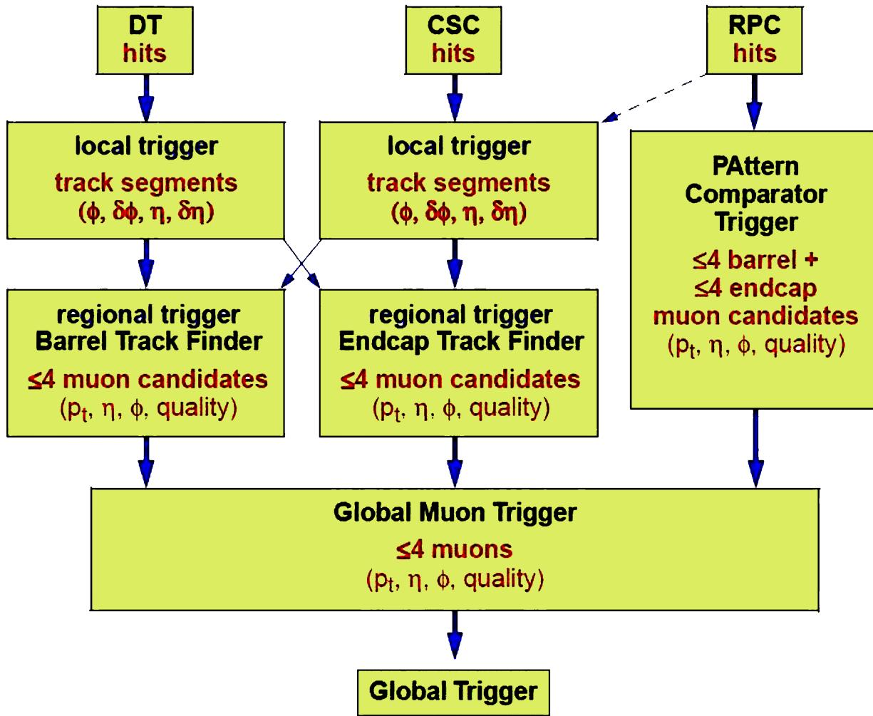
*All candidates are first sorted by quality, then by  $p_T$ . The L1 regional triggers deliver the 4 best muon candidates in the barrel and the 4 best muon candidates in the endcap to the global muon trigger (GMT).*
