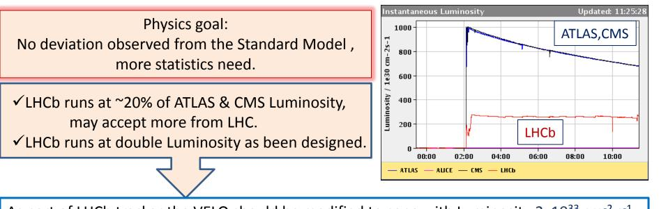
As part of LHCb tracker the VELO should be modified to cope with Luminosity  $2x10^{33}$  cm<sup>-2</sup> s<sup>-1</sup>
