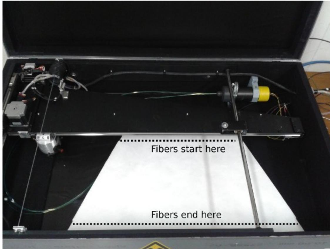
Test scintillator and fibers moving the Sr source on the scintillator surface
