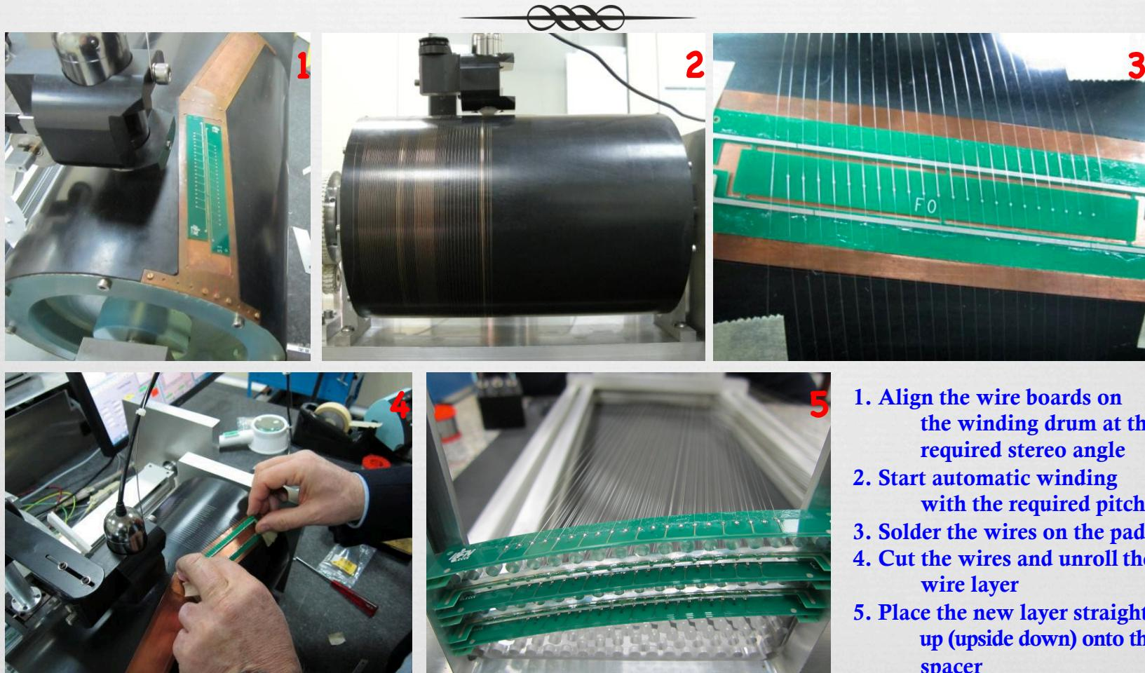
1. Align the wire boards on the winding drum at the required stereo angle
