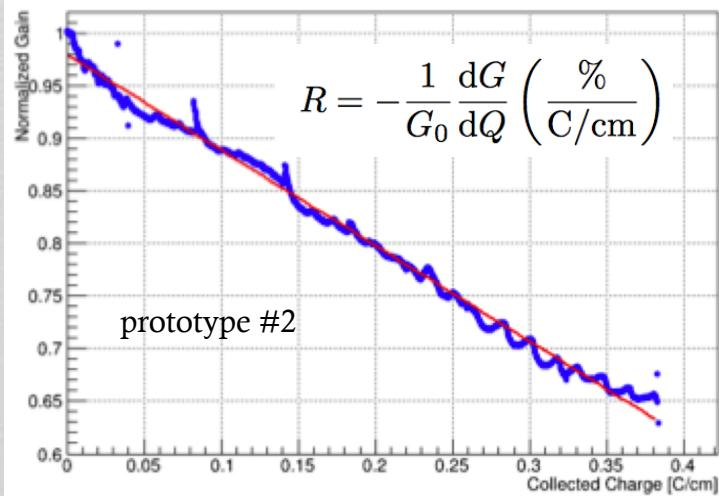
$\textcircled{1}$  @  $7 \times 10^7 \mu/\text{s}$  and  $10^5$  gas gain
