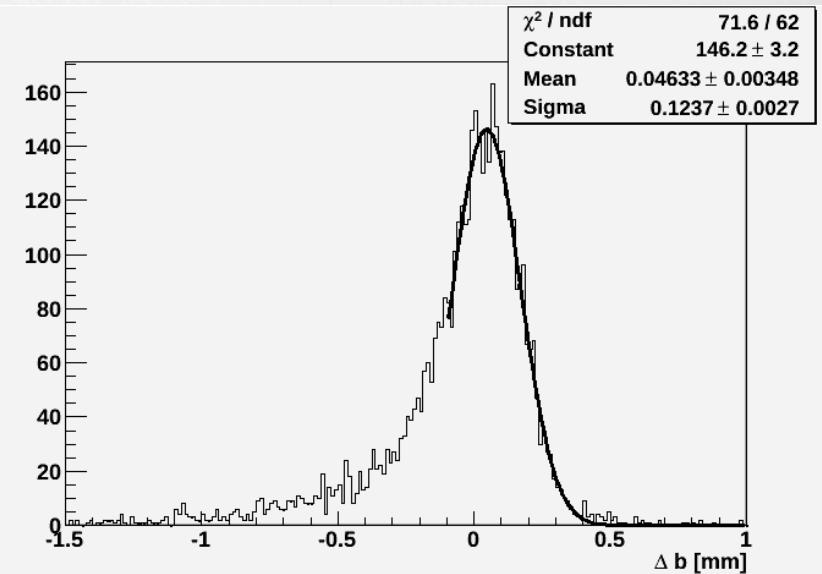
Average hit resolution  $\sigma_{\text{drift}} = 108 \pm 5 \mu\text{m}$
