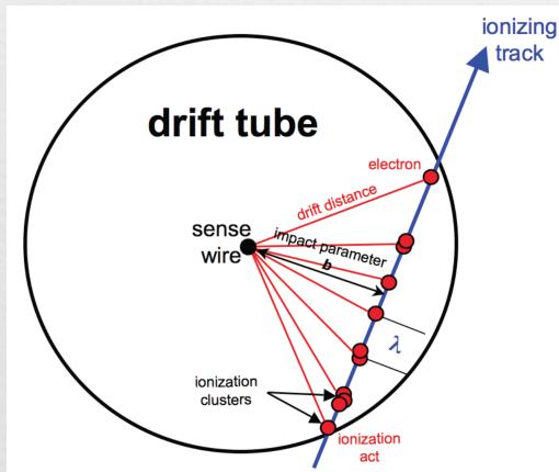
Recording the digitized information of all active sense wires in a drift chamber with full details (2 Gsa/s) may be a cumbersome task.
