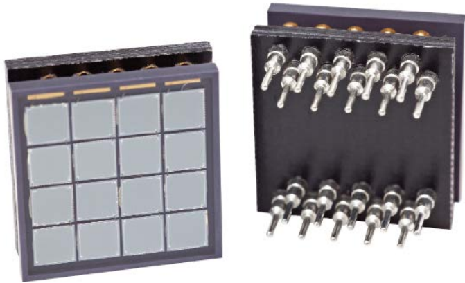
MPPC array for MAGIC telescope
