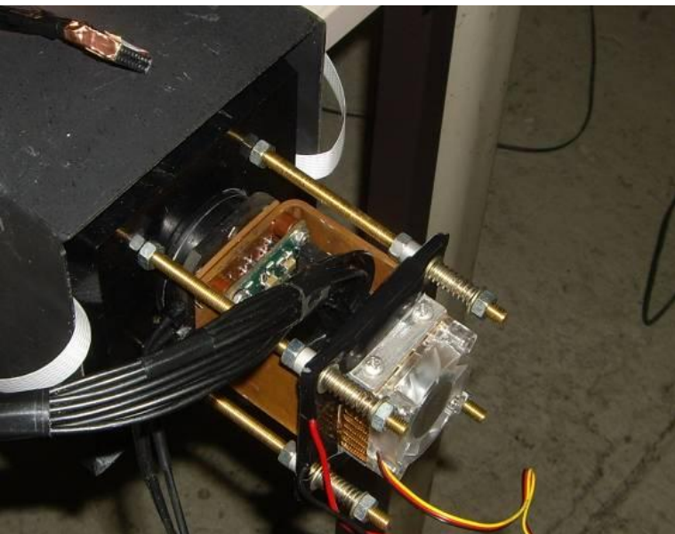
Sampling ADC front-end electronics designed and built by the group of Dr. S. Basylev
