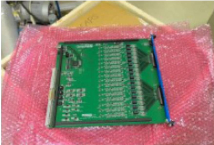
Shaper+DSP board for barrel
