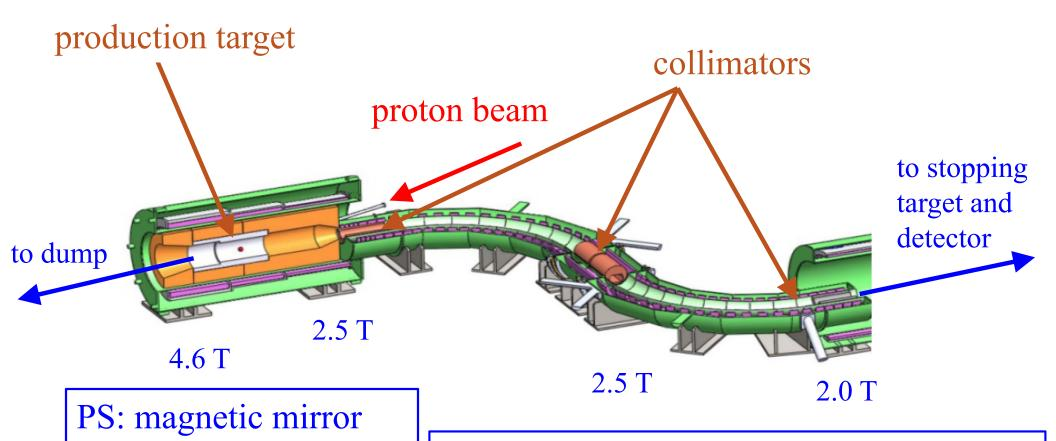
TS: negative gradient and charge selection at the central collimator
