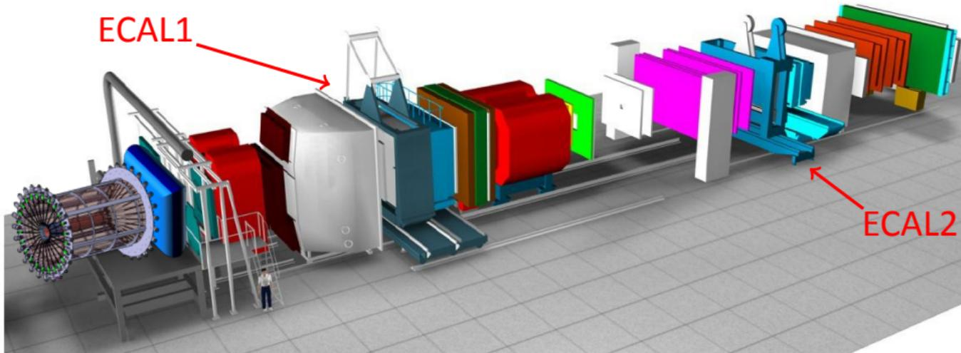
Two stage magnetic spectrometer for **large angular & momentum acceptance**
