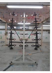
test elements of Pierre Auger mirror mirror of 13 m<sup>2</sup> at KIT, ROC=3.4m
