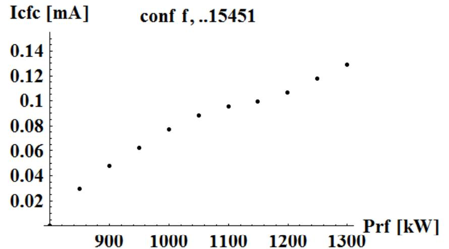
Beam current vs rf power for config 'f'
