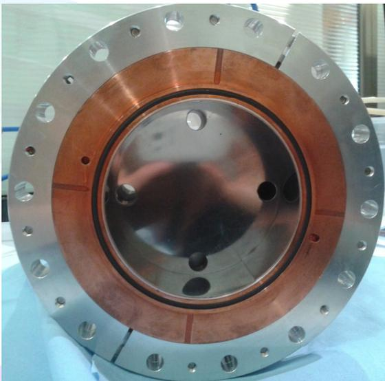
**Figure above: Rear cover and multipole covered by Mo liners; note a liner also protects O-ring**
