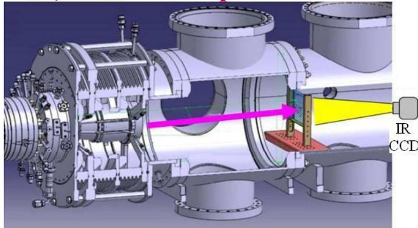
Figure: Cut view of NIO1 pumping cross, showing CFC tile
