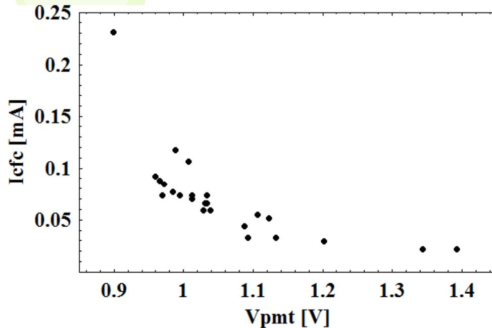
The puzzle of config 'e' : beam current increase with low luminosity ( $V_{pmt}$ ) at all control fixed, mainly  $P_k=1.2\text{kW}$ ,  $I_{pg}=10\text{ A}$ ,  $p_1=0.75\text{ Pa}$ ; the spontaneous or transient effect
