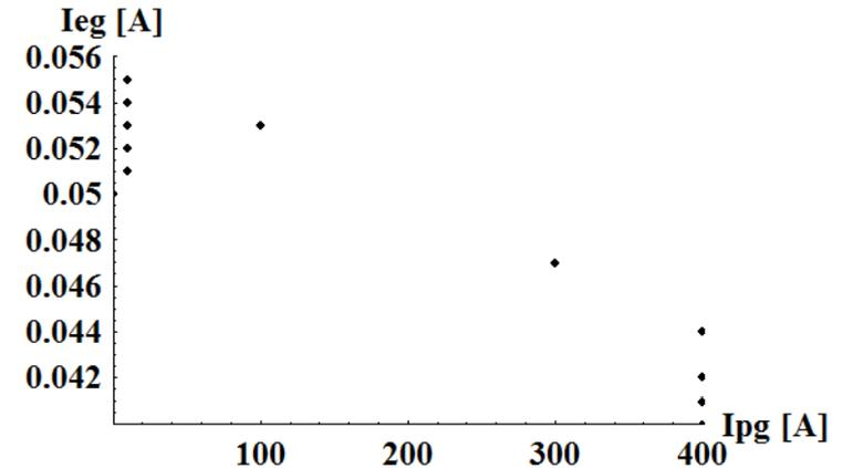
Beam current with  $p_1=0.4$  Pa for config 'e' and  $P_k=1.2$  kW similarly decreases with  $I_{pg}$ ,
