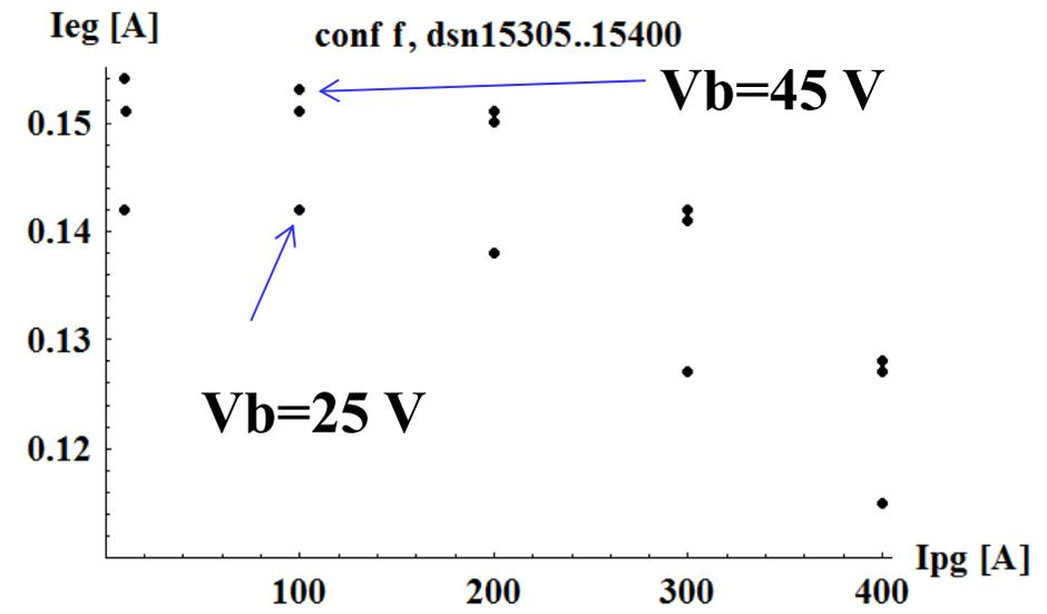
The coextracted electron current for Vb (bias voltage) and filter current for config 'f'; preliminary results seems more regular than for previous configurations
