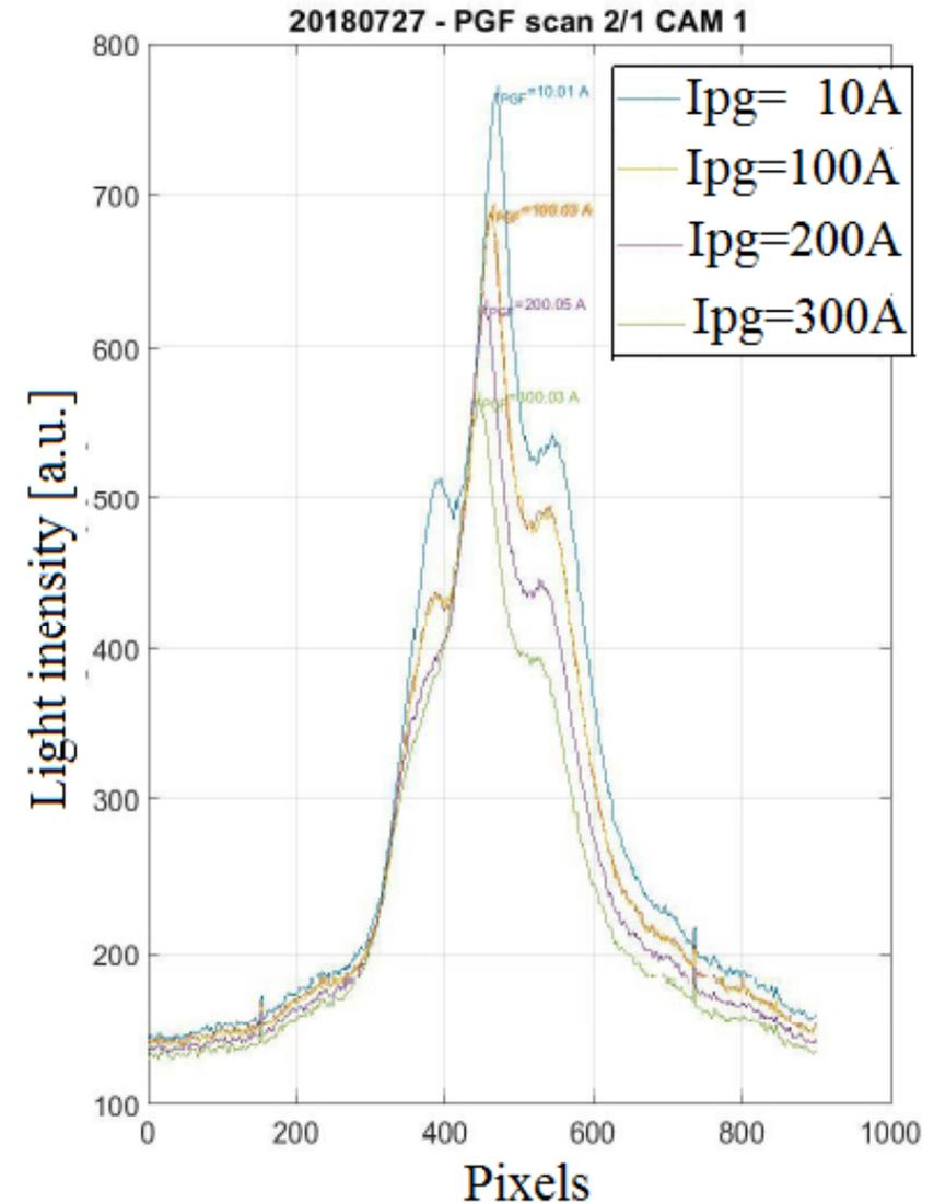
Some beam image and inferred profiles for several filter current
