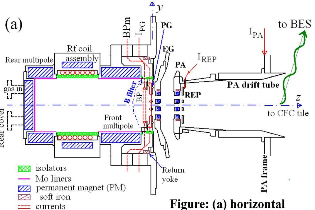
Figure: (a) horizontal zy section of NIO1 source and electrode; note filter position; (b) isometric view of NIO1 vacuum vessel
