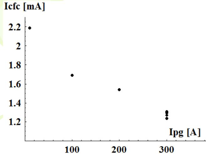
Beam current with  $p_1 = 0.75$  Pa for conf 'd2' decreases with filter  $I_{pg}$
