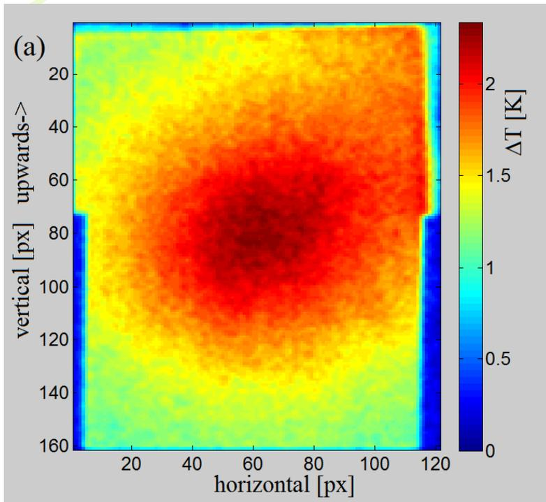
(a) Temperature rise  $\Delta T$  on the CFC tile in 150 s, 1 px = 0.75 mm;
