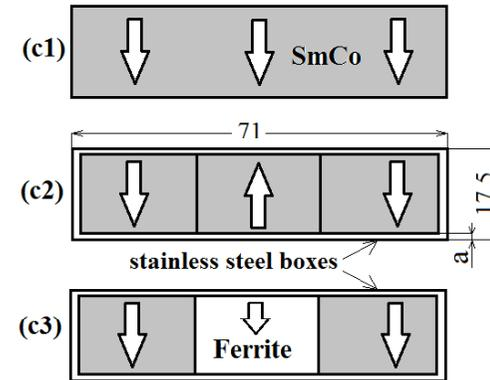
**Figure: simple or simply modified multipole bars: (c1) solid block; (c2) central piece is reverse, note containing box thickness; (c3) central piece is different**
