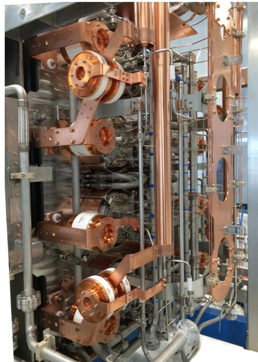
**View of SPIDER (behind-side); note capacitor (white) and rf connection (shiny solid copper)**
