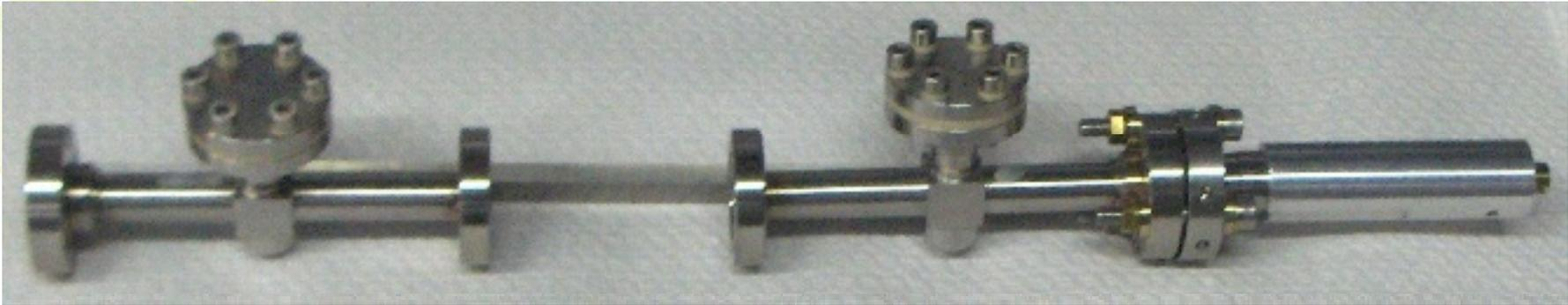
**4.3) The flange for CRD installation in NIO1, integrating shutter and micrometric mirror movements; built July 2018; under installation**
