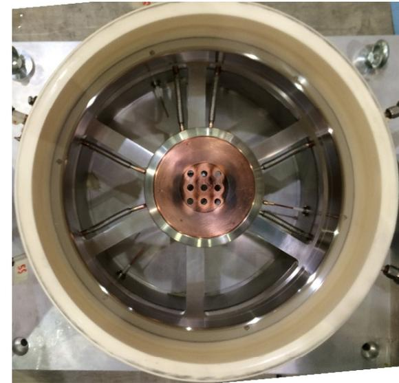
**May 2017 disassembly config 'c' = the old EG: note burns with a zigzag patterns**
