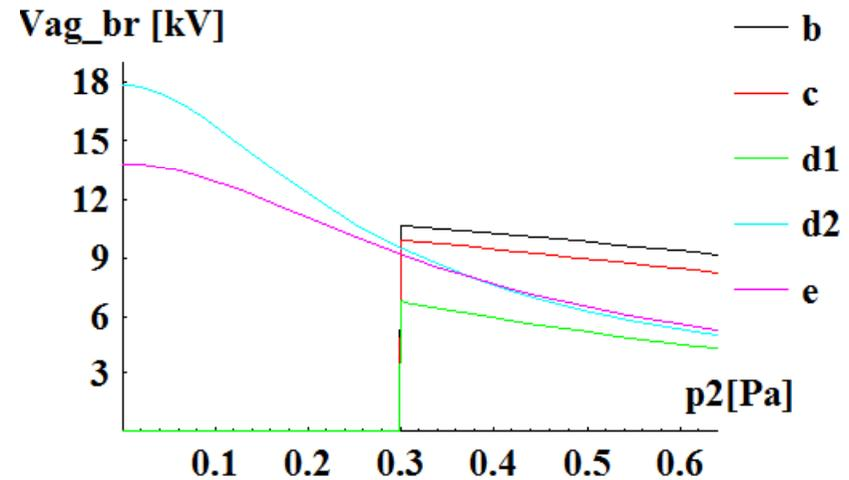
Trends of Breakdown voltage vs vessel pressure for H2 for config b-e
