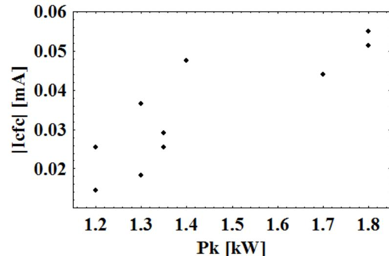
Beam current with  $p_1=0.4$  Pa for config 'e' increase with  $P_k$ , at least up to 1.5 kW,
