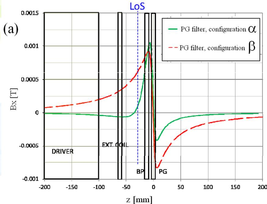
Figure: (a) field  $B_x$  vs  $z$ , with  $I_{PG}=100$  A (b) old circuit; (c) circuit using C-conductors
