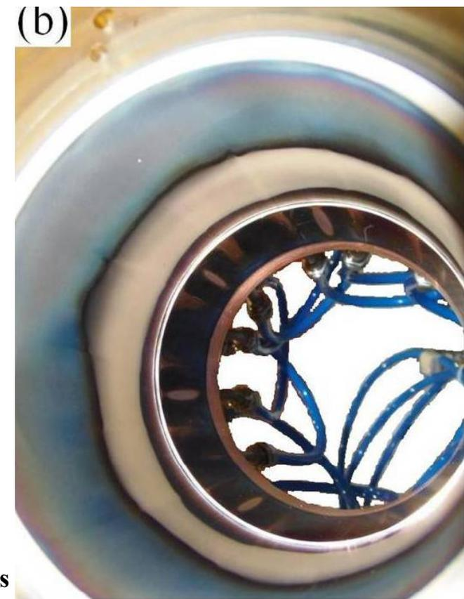
**(b) OLD STATUS OF source walls and rf window:** After operation at rf power 1.7 kW, a vacuum loss appeared (probably for elastic bolts unbalanced loosening, possible with vibration; finer mechanical adjustments are in progress). The opening of the source makes some observation possible: some wall deposit is apparent ; two conductive rings appears at rf window ceramics ends. This suggests periodical inspection of source (opening rear cover) and use of Mo liners
