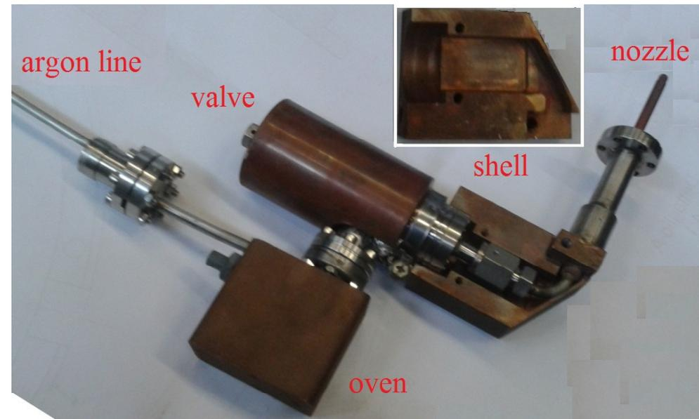
**Figure: design of the second Cs evaporator for NIO1, using solid pellets**
