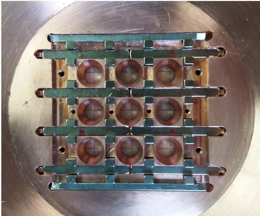
The new extraction grid can hold either standard CESM configuration or CESM+ADCM configuration (Chitarin et al RSI 2013), with many variants (Cavenago and Veltri, PSST 2014)
