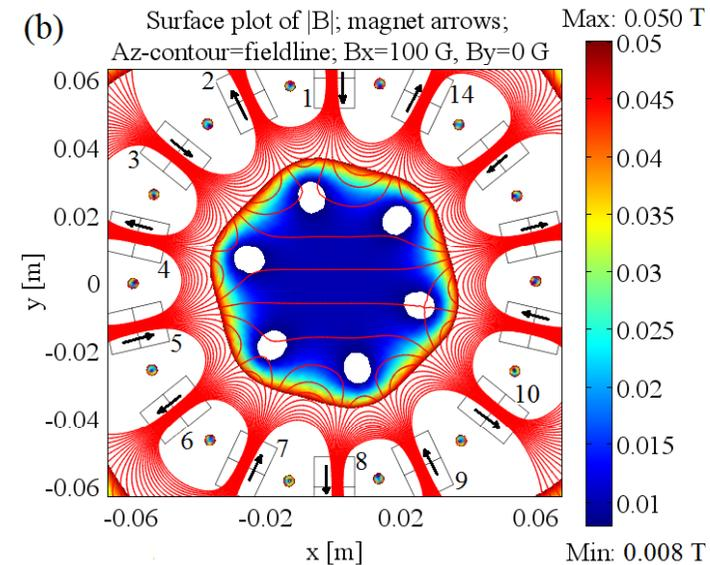
**2D concept of isobars for config c style and config f style (Cavenago, Baltador, Veltri, ICIS2017, in press); white island are confinement leak. Note regular hexagon in config 'f' concept. Confirming 3D simulations mostly completed to appear soon (Baltador et al)**
