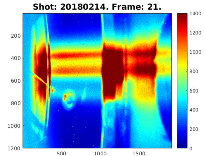
**NIO1 Beams, up to 4 mA (April 2017), view from down; note 3 rows of beamlet, with spacing difference possibly due to old EG magnets.**
