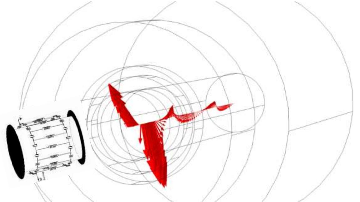
Radial electric field vector along the z-axis
