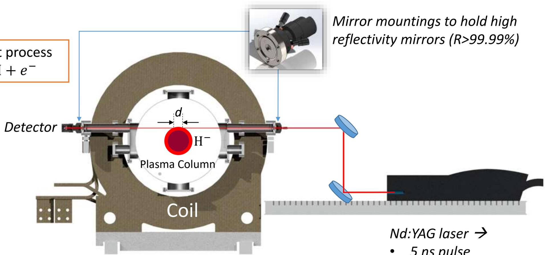
The extinction time of light in the optical cavity depends on medium absorbance
