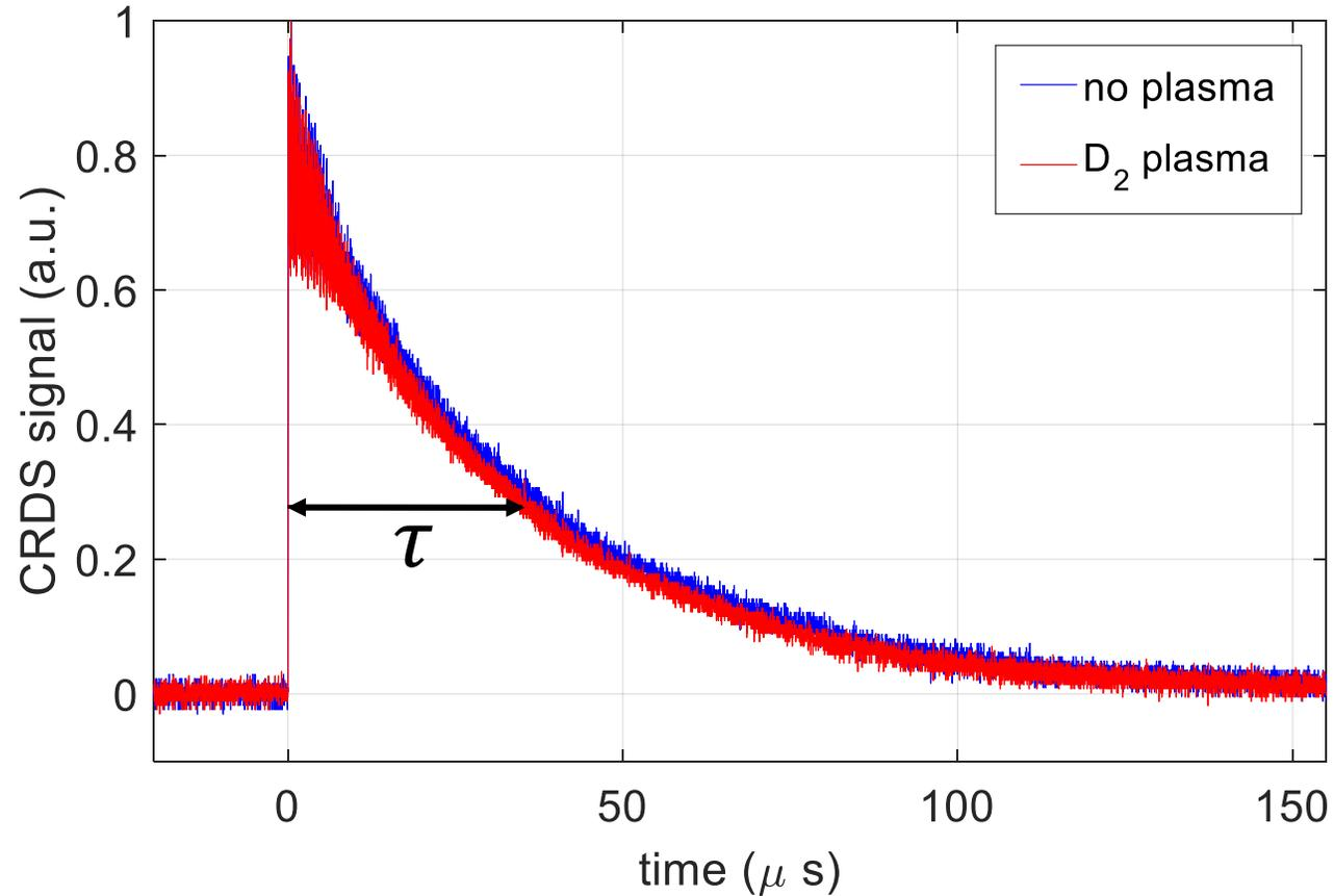
*Typical decay signals in two conditions: in vacuum (no plasma) and in a D<sub>2</sub> plasma*
