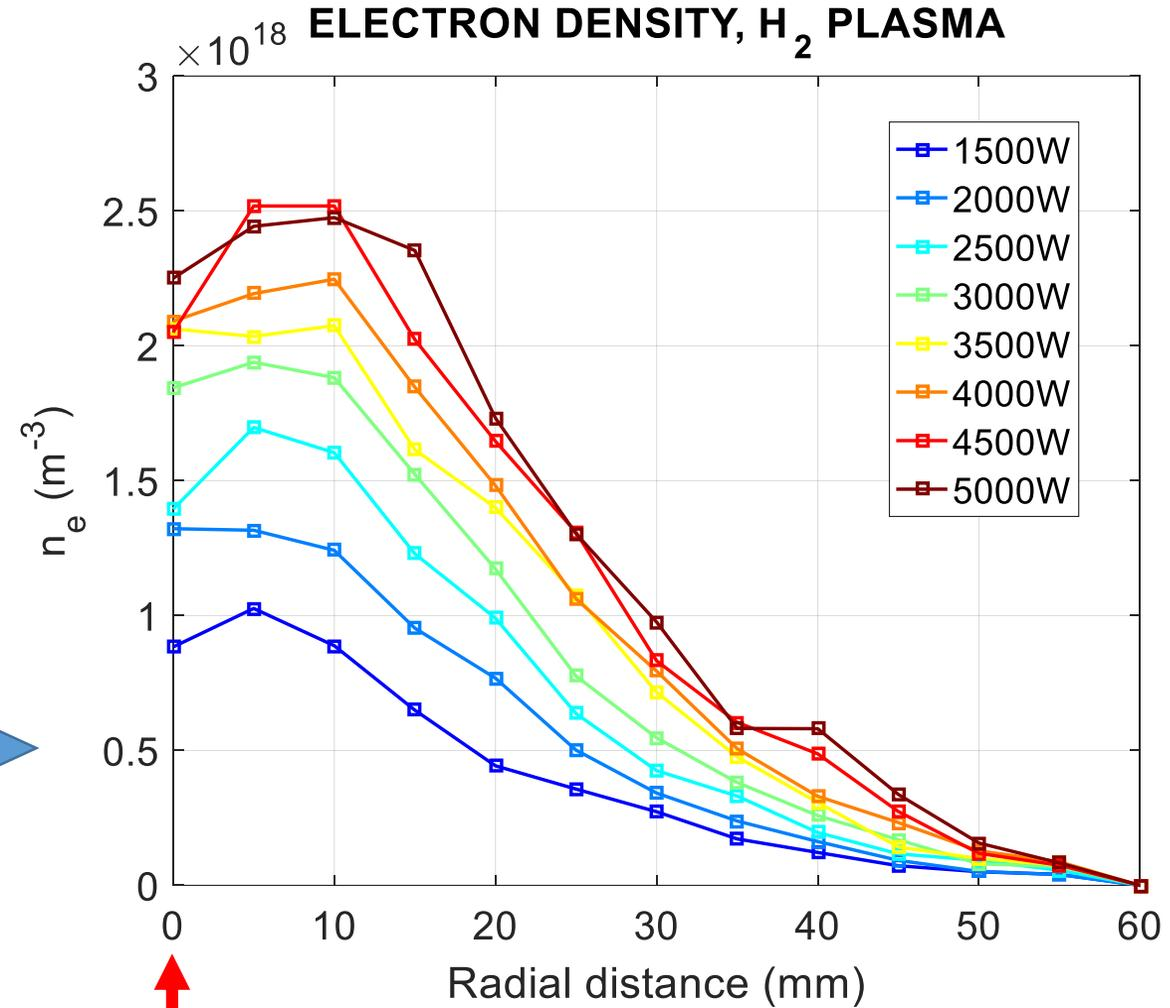
Electron density profiles are calibrated with a 100 GHz microwave interferometer
