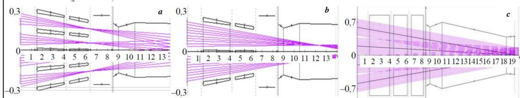
Beamlet focusing scheme for the DEMO-FNS injector: horizontal focusing - four channels (a), two channels (b); Vertical focusing is common for both figure (c). Vertically, within each group, the beamlet axis is parallel
