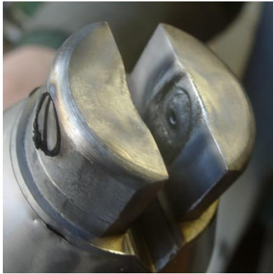
Cathode erosion after 12 month work
