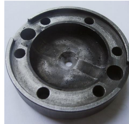
Moly film deposition to anode cover after 160 hours run
