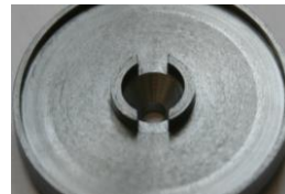
Collar around the emission aperture at the anode cover
