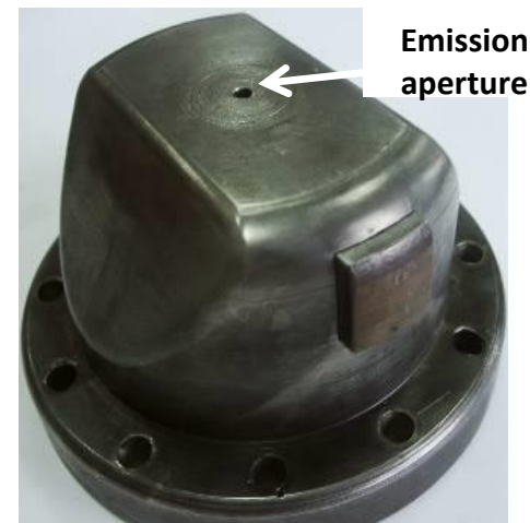
Anode body with emission aperture
