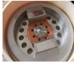
Magnets with yoke are placed inside HV ceramics
