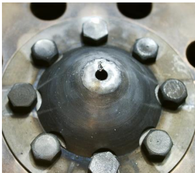
Accelerated Electrode melting by electrons
