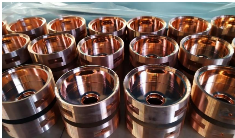
Cells of the accelerating structure
