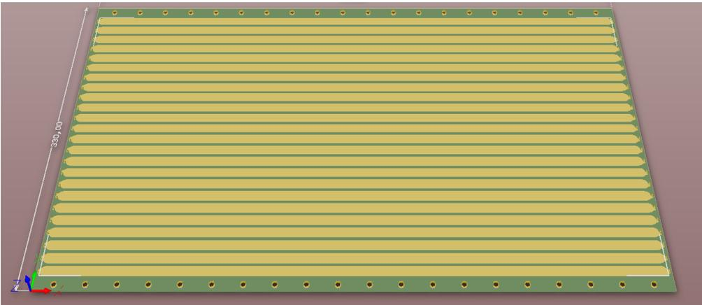
Inner readout board with strips
