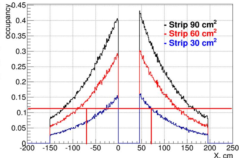
Mean particle flux in different regions of the TOF surface
