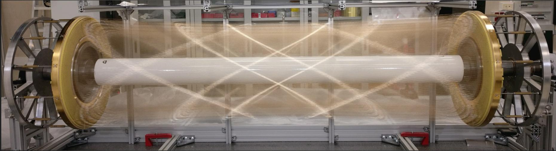
A unique volume, high granularity, all stereo, low mass cylindrical drift chamber, co-axial to B.
