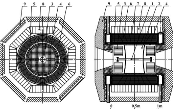
1 – Be beam pipe, 2 – drift chamber, 3 – BGO calorimeter, 4 – Z-chamber, 5 – superconducting solenoid, 6 – LXe calorimeter, 7 – TOF, 8 – CsI calorimeter, 9 – yoke
