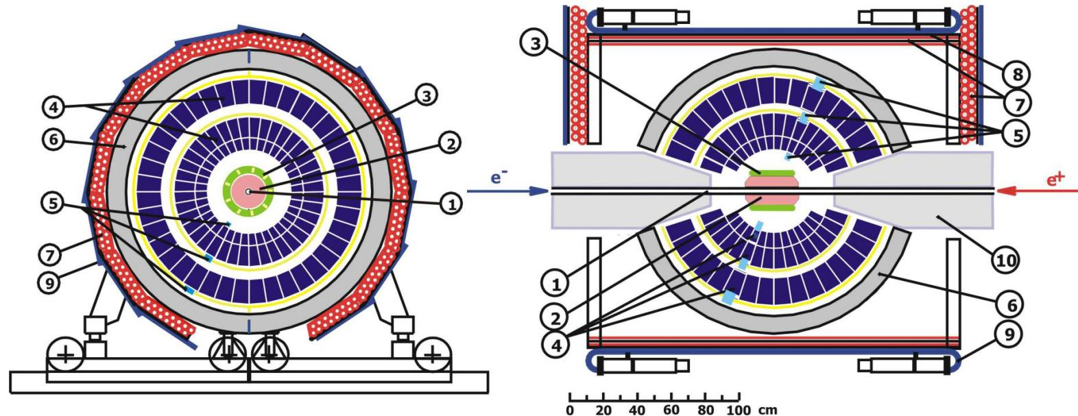
1 – beam pipe, 2 – tracking system, 3 – aerogel Cherenkov counters , 4 – NaI(Tl) crystals, 5 – phototriodes, 6 – iron muon absorber, 7–9 – muon detector, 10 – focusing solenoids.
